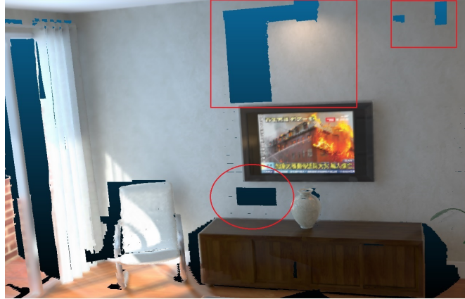
Figure 4.8: Undesirable holes in reconstructed model from ICL-LR2 trajectory.
