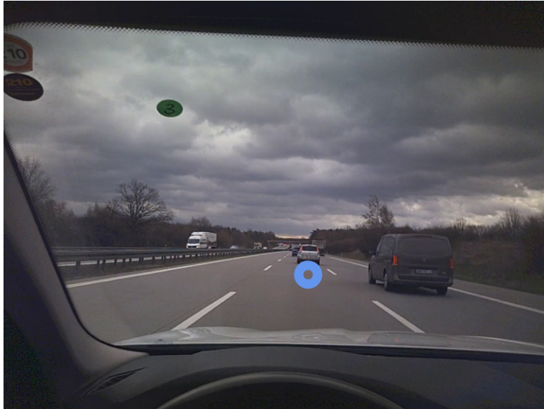
Figure 6.2: The first person view from the participant who wears the SMI glasses is driving on the highway, where the blue point is the fixation monitored by eye-tracker.
