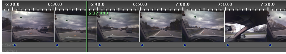
(a) A screen shot taken from the software used to process eye-tracking data, where the blue points are the messages from PC used to record CAN signals carrying Unix timestamps.
