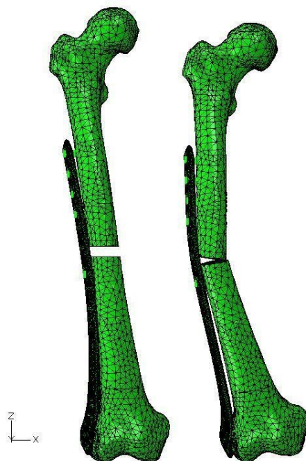
Figure 2-15: Collapse of the fracture gap with contact of the proximal and distal segments for a 10 mm diaphyseal gap under walking loads without additional support within the fracture gap.
