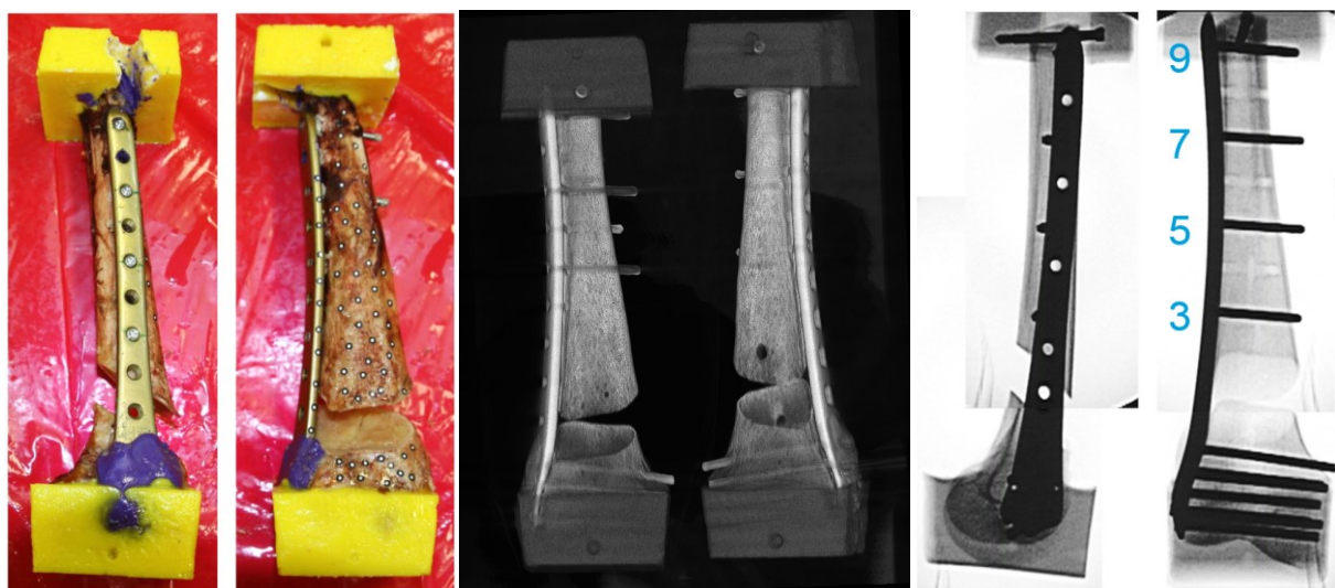
Figure 2-28: From left to right: Example of validation specimen of a distal femur with lateral plate fixation, embedded in PMMA (with purple clay to allow free plate motion). CT-images were obtained after testing to verify integrity and for modelling. Fluoroscopic images show the screw position (number of holes 9,7,5,3 marked) and the empty screw holes of previous testing.
