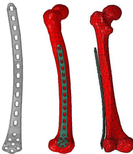
Figure 2-16: Plate placement is not trivial as there is no universal algorithm. Surgical techniques vary and thus plate placement may vary strongly. We tried to place the plate with a small distance between the plate and the bone (clearance) to allow for free plate bending. However, this bone-plate distance should remain small over the whole plate length to avoid excessively long free bending lengths of individual screws. Furthermore, excessive distance of the plate from the bone results in decreased plate strength Ahmad et al. (2007).
