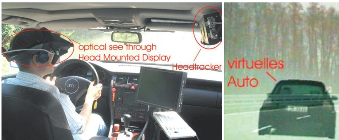
Bild 2-9: Vehicle in the Loop [73]
