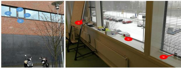
(a) Location of sensors on the inside and outside of the workplace.
