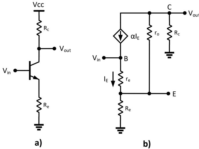
**Figure 2.2:** a) Schematic of a single-ended common-emitter amplifier with emitter resistance. b) HBT replaced by the T model in the amplifier schematic.
