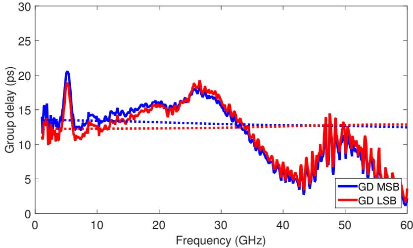
**Figure 4.17:** S-parameters results (group delay). Comparison between post-layout simulation (dashed) and measurements (solid).
