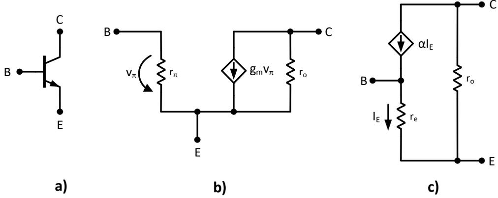
**Figure 2.1:** Small signal model of the HBT. a) HBT symbol with 3 terminals b) the hybrid- $\pi$  model and c) the T model
