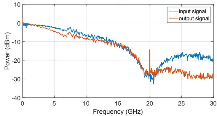
**Figure 3.19:** Spectrum of the optical output in a PAM-4 transmission ( $2^7-1$  PRBS) at 20 Gbaud (40 Gb/s). The spectrum of the input signal is also plotted.
