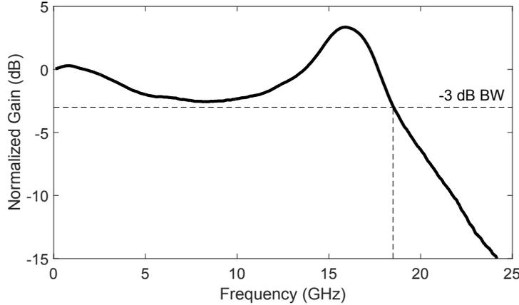
**Figure 3.16:** Electro-optical bandwidth measurement with normalized gain with reverse bias of 1.5 V applied to the MZM.
