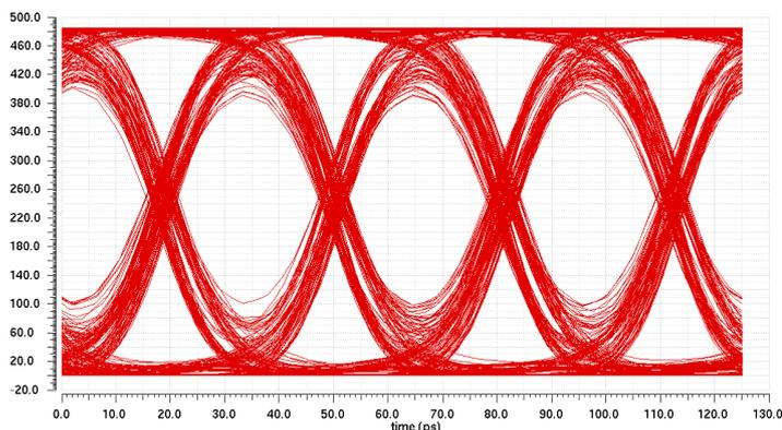
**Figure 3.14:** Simulated optical output eye-diagram transmitting OOK signal at 32 Gb/s, using the co-simulation.
