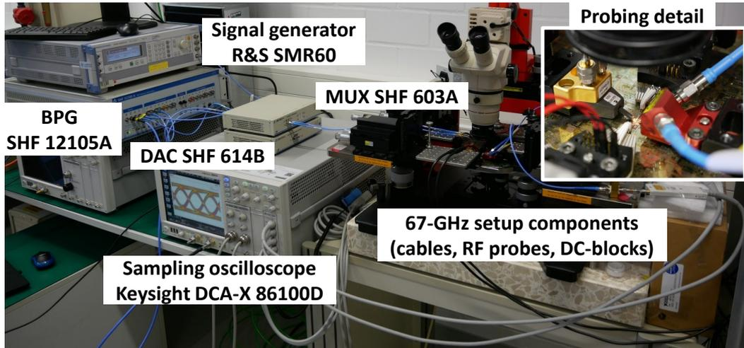
**Figure 5.16:** Experimental setup for on-wafer time-domain measurements. The inset shows the magnified picture of the probing setup.
