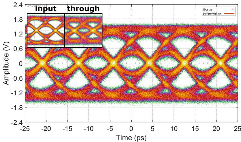
**Figure 5.19:** Differential output eye-diagram OOK 120 Gb/s with  $3 V_{ppd}$  (input  $0.9 V_{ppd}$ ). Measured eye amplitude is 1.775 V, jitter peak-to-peak is 4.0665 ps and jitter rms is 571.5 fs. The insets show the input eye-diagram and the measured eye-diagram with a through structure.
