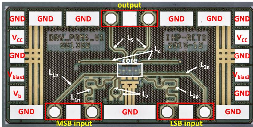
Figure 4.15: Chip microphotograph.
