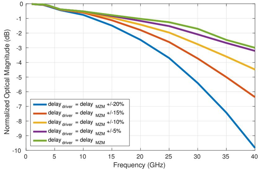
**Figure 2.22:** Impact on the MZM bandwidth of the velocity mismatch between electrical and optical waves in the segmented driving approach.
