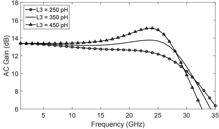
Figure 3.7: Simulation of the contribution of the inductor L3 to the driver frequency response.
