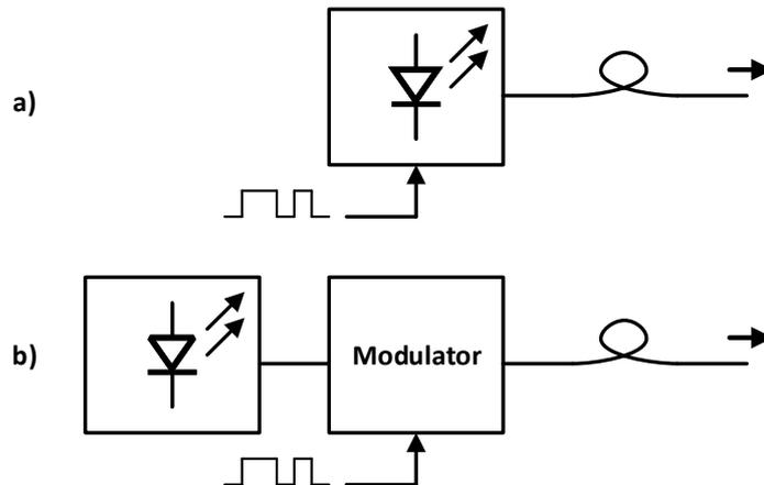
**Figure 1.2:** Types of optical transmitters. a) Direct modulation b) External modulation.
