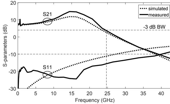
**Figure 3.9:** Driver S-parameters results. Comparison between post-layout simulation and measurements.
