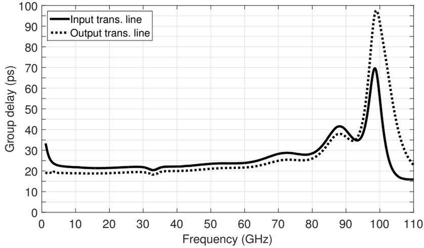
**Figure 5.2:** Simulation of the group delay of input and output transmission lines.
