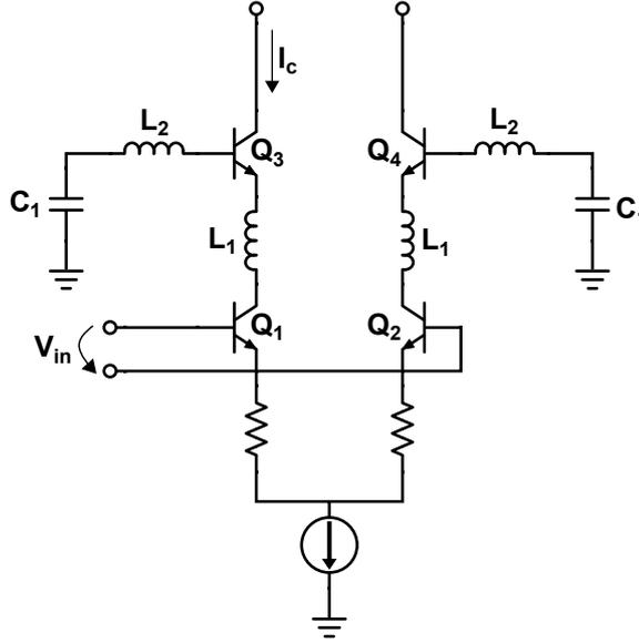
**Figure 5.4:** Simplified schematic of the gain cell.
