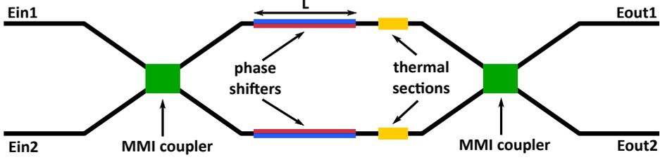
**Figure 2.21:** Block diagram of the MZM optical components implemented in the co-simulation.
