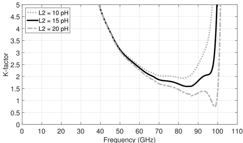
**Figure 5.5:** K-factor simulation for different values of  $L_2$ .
