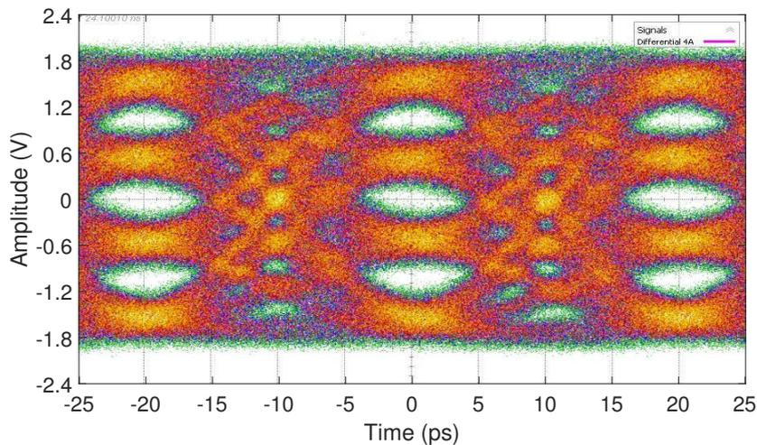
**Figure 4.19:** Measured PAM-4 differential eye-diagram of the driver output at 50 Gbaud (100 Gb/s) using PRBS31 at the input.
