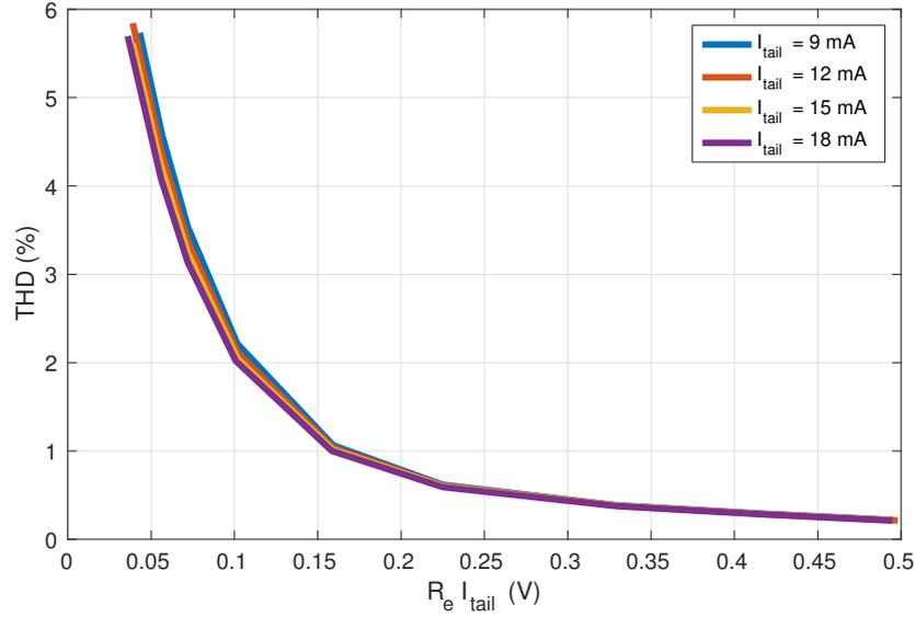
**Figure 2.6:** THD versus  $R_e I_{tail}$  for different  $I_{tail}$  values ( $g_m$  change).
