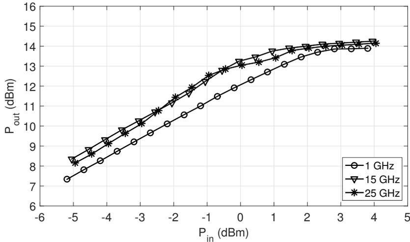
**Figure 5.15:** Measured output power ( $P_{out}$ ) over input power ( $P_{in}$ ) for different frequency values.
