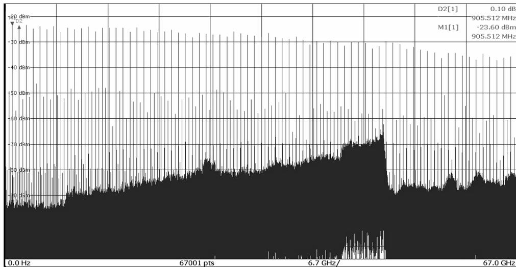
**Figure 5.31:** Measured spectrum of the output pattern at 115 Gb/s with tone spacing of 905.512 MHz.
