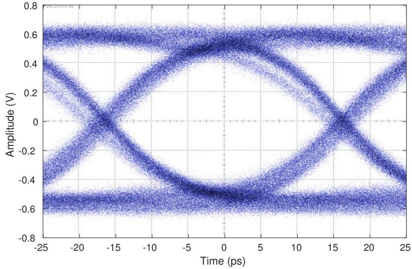
**Figure 4.5:** Differential output eye-diagram at 32 Gb/s. Signal is attenuated by 10 dB at the input of the oscilloscope. Input amplitude is limited to 1.2 Vppd.
