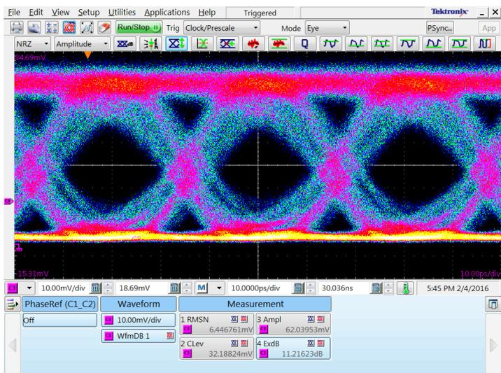
**Figure 3.15:** Measured optical output eye-diagram transmitting OOK signal at 32 Gb/s using  $2^{31}-1$  PRBS without pre-emphasis.
