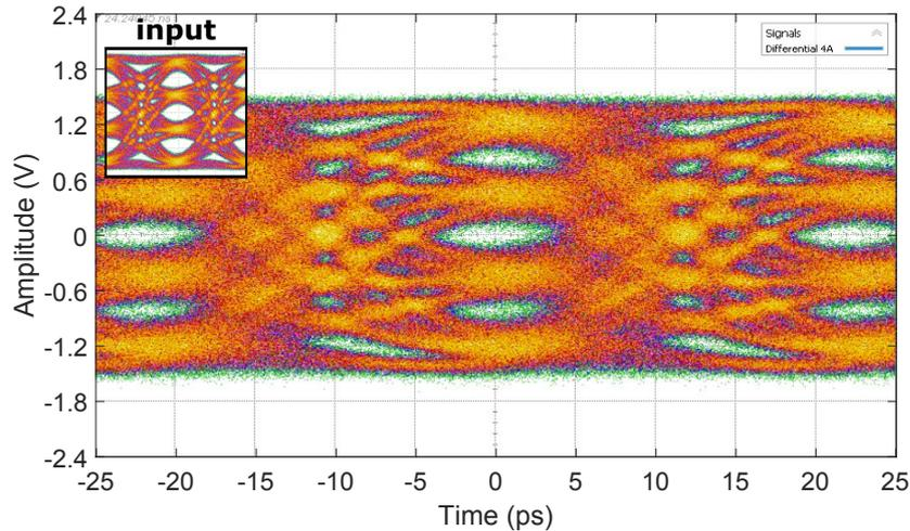
**Figure 5.20:** Differential output eye-diagram PAM-4 45 Gbaud (90 Gb/s) with  $3 V_{\text{ppd}}$  (input  $0.9 V_{\text{ppd}}$ ), without pre-emphasis. The inset shows the input eye-diagram.
