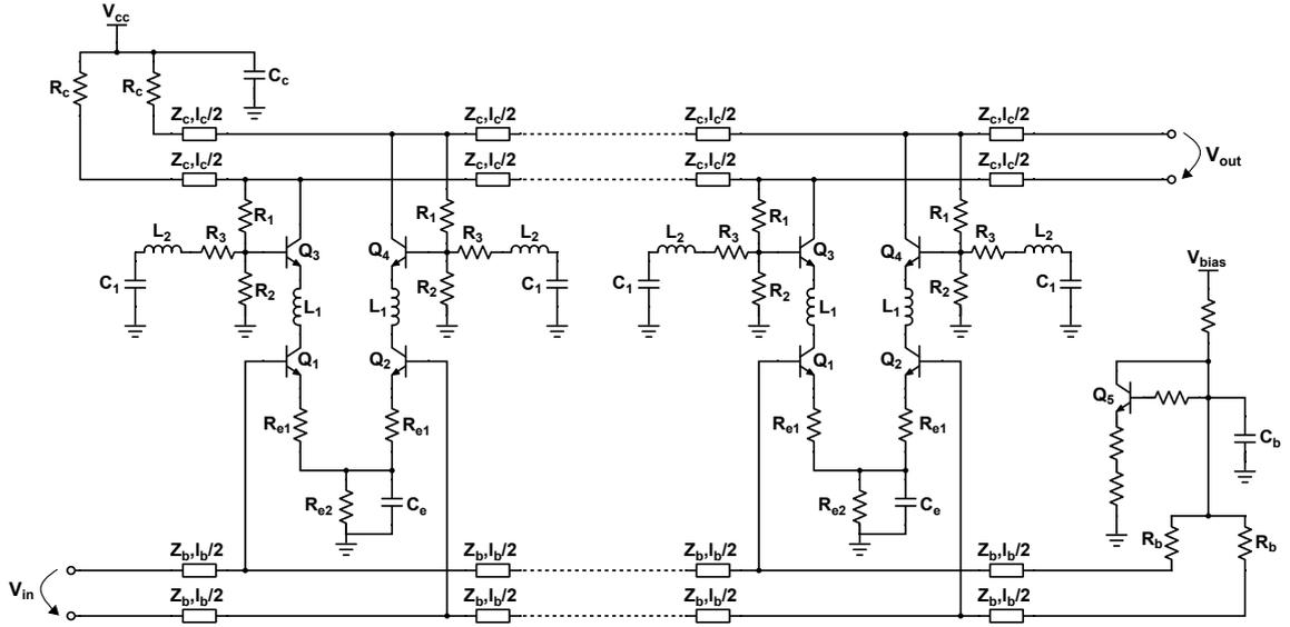
Figure 5.6: Full circuit schematic.
