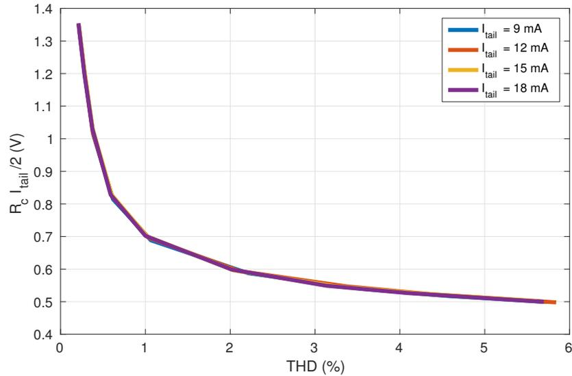
**Figure 2.7:** Voltage headroom ( $R_c I_{tail}/2$ ) over THD values for different  $I_{tail}$  values ( $g_m$  change).
