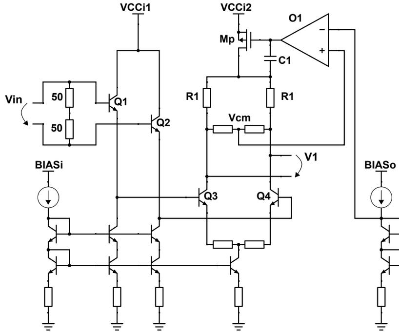
Figure 3.3: Driver input stage schematic.
