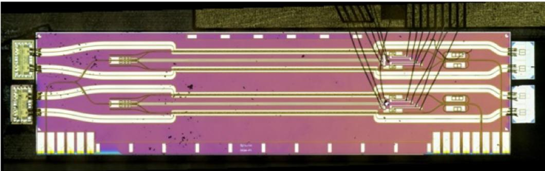
**Figure 4.7:** Electro-optical module comprising two 25- $\Omega$  IQ drivers and a dual-IQ optical modulator.
