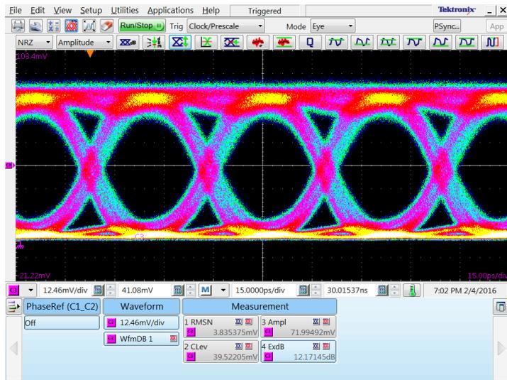
**Figure 3.13:** Measured optical output eye-diagram transmitting OOK signal at 28 Gb/s using  $2^{31}-1$  PRBS without pre-emphasis.
