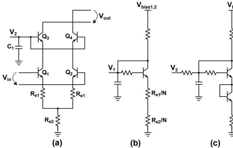
Figure 4.14: Stages schematics. a) amplifier b) input base bias and c) cascode base bias.
