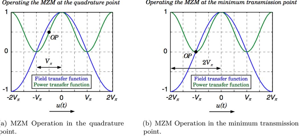
**Figure 2.14:** MZM Operation in the quadrature point and the minimum transmission point [8].
