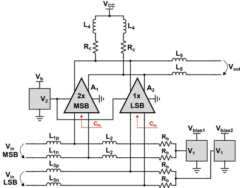
Figure 4.13: Schematic of the PAM-4 driver.
