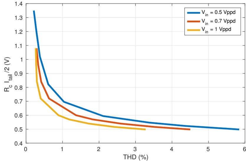
**Figure 2.10:** Voltage headroom ( $R_c I_{tail}/2$ ) over THD values for different input amplitudes.
