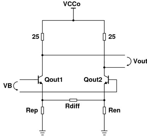
**Figure 4.1:** Detailed schematic of the driver output stage.
