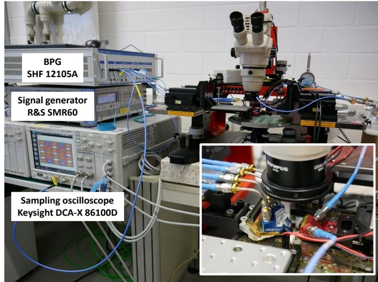
**Figure 4.20:** Experimental setup for on-wafer PAM measurements. The inset shows the magnified picture of the probing setup.
