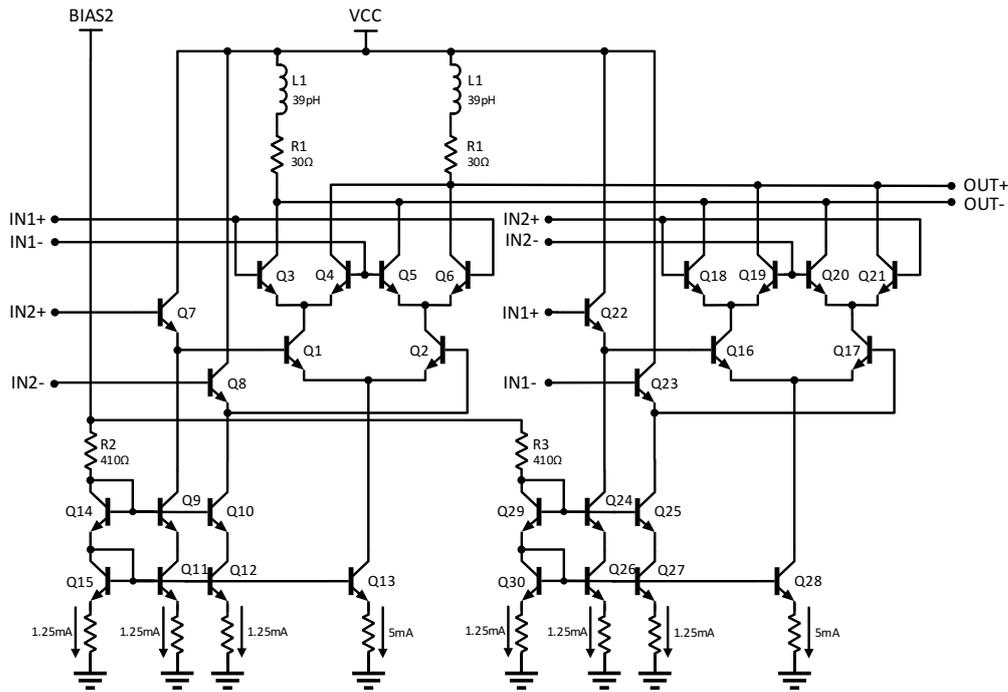
Figure 5.27: Schematic of the full-rate XOR gate (asynchronous).
