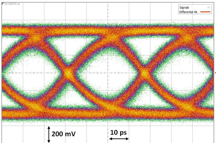
**Figure 4.12:** Measured differential eye-diagram at 28 Gb/s.
