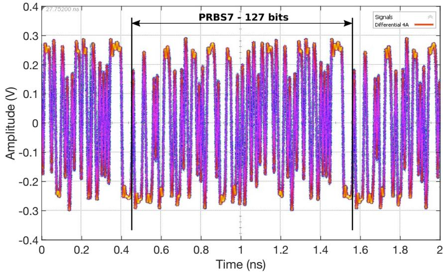
**Figure 5.30:** Measured differential output signal, showing the data pattern of the generated PRBS at 114.3 Gb/s.
