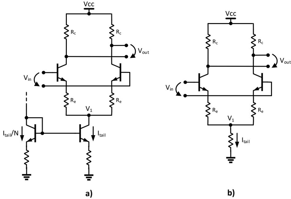
**Figure 2.5:** a) Differential pair amplifier with current mirror and b) with resistive current source.
