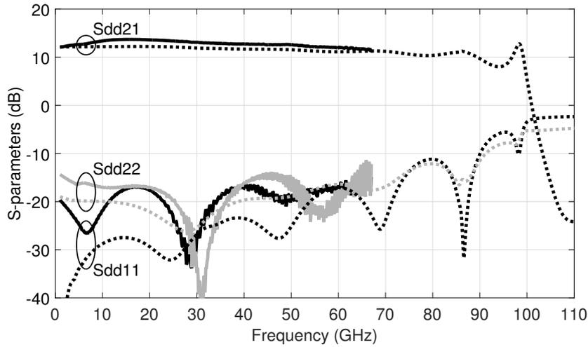
**Figure 5.11:** Differential S-parameters results (gain and return loss). Comparison between post-layout simulation (dashed) and measurements (solid).
