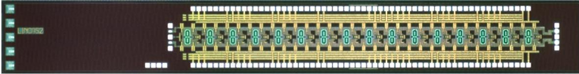
**Figure 3.26:** Chip microphotograph of the second generation optical transmitter.
