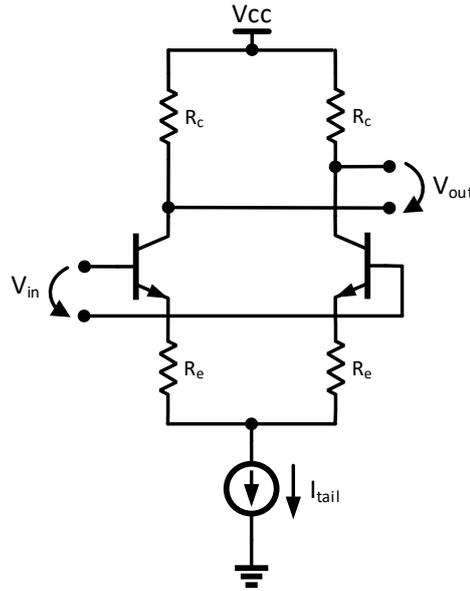
**Figure 2.3:** Schematic of a differential pair amplifier with emitter degeneration.
