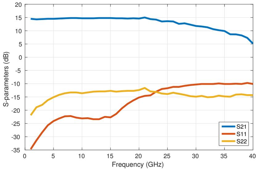
Figure 4.4: S-parameter measurements of the linear driver for 25- $\Omega$  MZMs.
