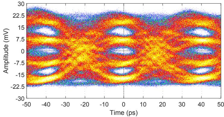
**Figure 3.21:** Measured optical output eye-diagram transmitting PAM-4 signal at 25 Gbaud (50 Gb/s) using  $2^7-1$  PRBS without pre-emphasis.
