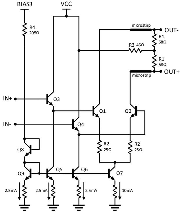
**Figure 5.25:** Schematic of the clock buffer.
