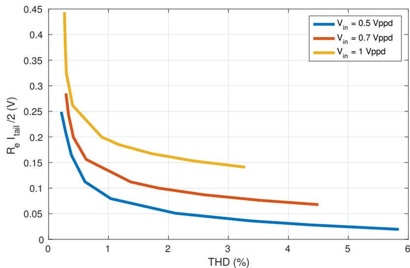
**Figure 2.11:** Voltage drop in  $R_e$  ( $R_e I_{tail}/2$ ) over THD values for different input amplitudes.
