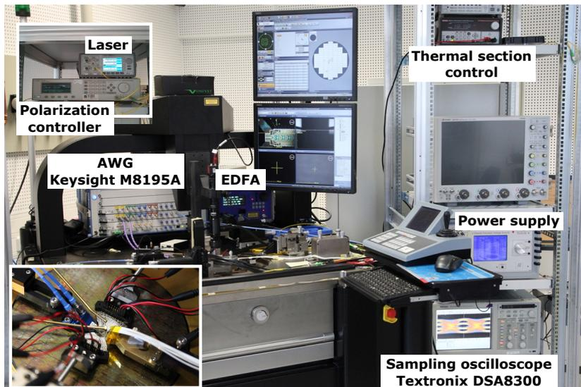
**Figure 3.23:** Experimental electro-optical setup for on-wafer PAM measurements using an AWG at the input. A magnified picture of the probing is also shown in the bottom-left corner.
