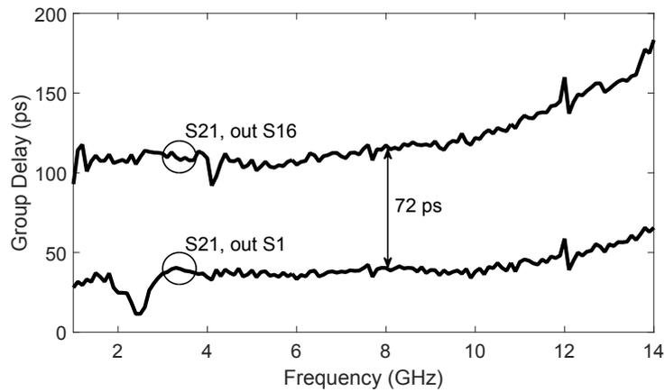
Figure 3.11: Group delay from the input to the output of the 1st segment and from the input to the output of the 16th segment of the driver.
