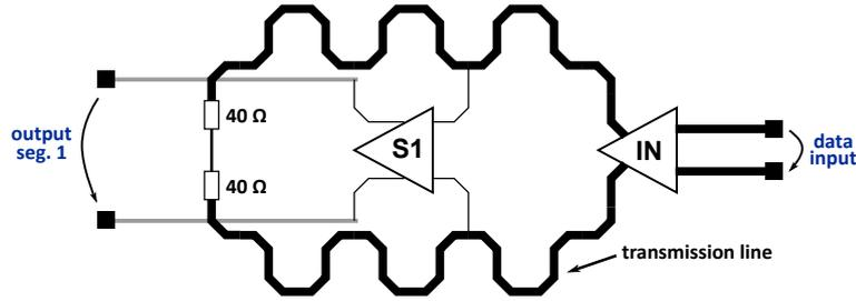
**Figure 3.8:** Block diagram of the single-segment variant.
