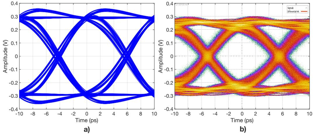
**Figure 5.28:** a) Simulated differential output eye-diagram at 100 Gb/s. b) Measured differential output eye-diagram at 100 Gb/s. The SNR has a value of 7.94 dB, the eye width is 7.63 ps, the eye height is 289 mV and the jitter rms value is 501.6 fs. The acquisition count number is 505.
