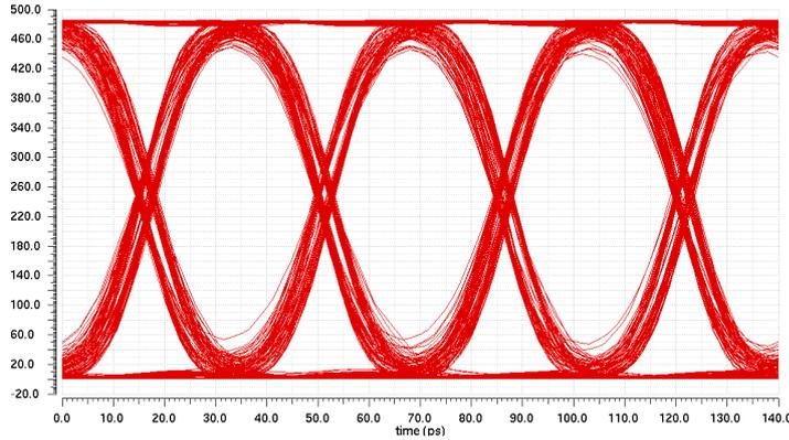
**Figure 3.12:** Simulated optical output eye-diagram transmitting OOK signal at 28 Gb/s, using the co-simulation.
