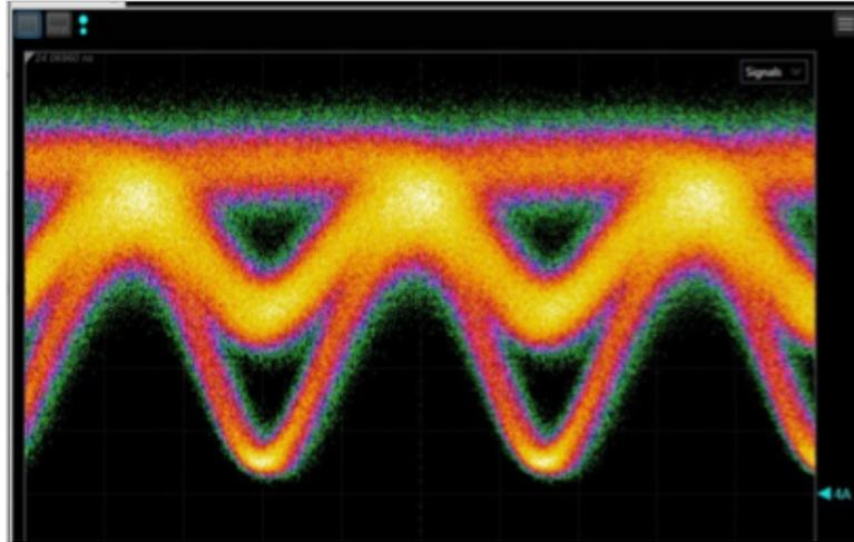
**Figure 4.8:** Optical magnitude at the output of one of the IQ modulator arms of the generated QPSK signal at 25 Gbaud.
