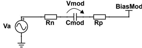
**Figure 2.20:** Electrical lumped model of the MZM phase shifter segment.
