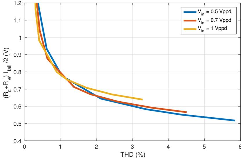
**Figure 2.12:** Sum of voltage drop in  $R_c$  and  $R_e$  over THD values for different input amplitudes.
