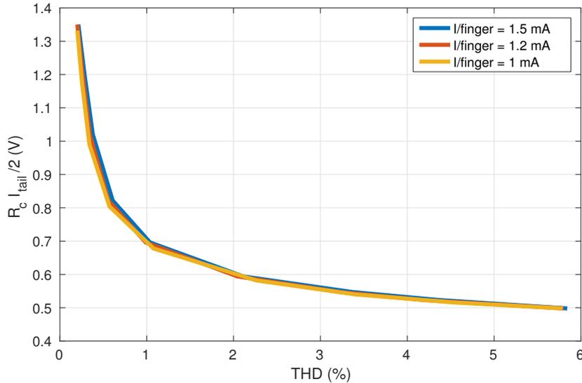
**Figure 2.9:** Voltage headroom ( $R_c I_{tail}/2$ ) over THD values for different current densities per HBT finger.
