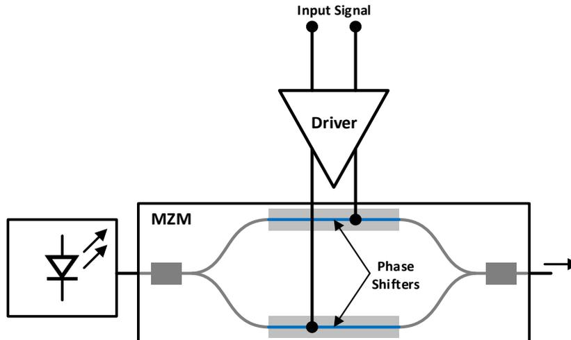
**Figure 2.16:** Lumped Electrode MZM driving scheme.
