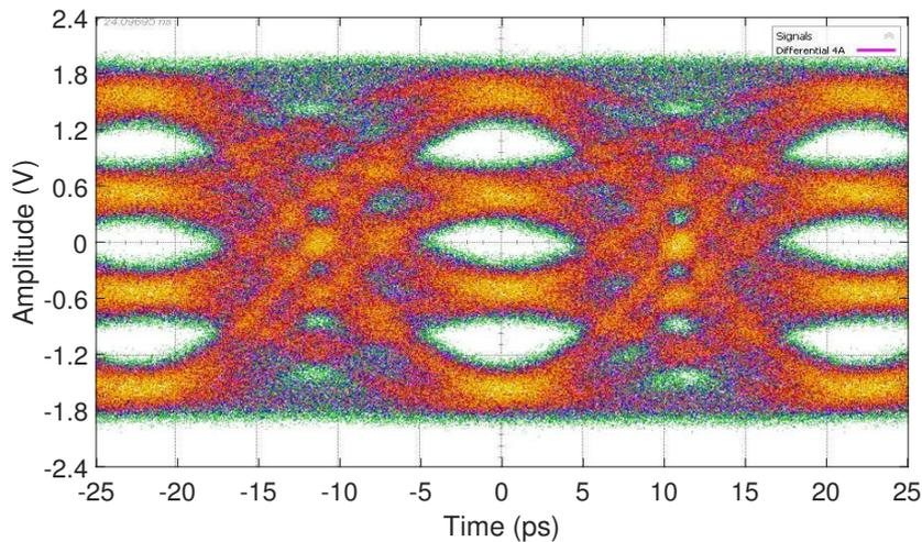
**Figure 4.18:** Measured PAM-4 differential eye-diagram of the driver output at 45 Gbaud (90 Gb/s) using PRBS31 at the input.
