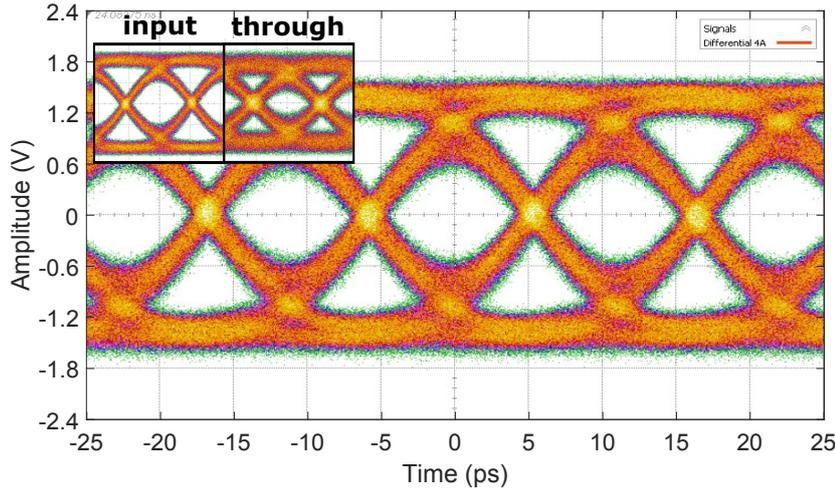
**Figure 5.18:** Differential output eye-diagram OOK 90 Gb/s with  $3 V_{ppd}$  (input  $0.9 V_{ppd}$ ). Measured eye amplitude is 2.123 V, jitter peak-to-peak is 3.4 ps and jitter rms is 609.5 fs. The insets show the input eye-diagram and the measured eye-diagram with a through structure.
