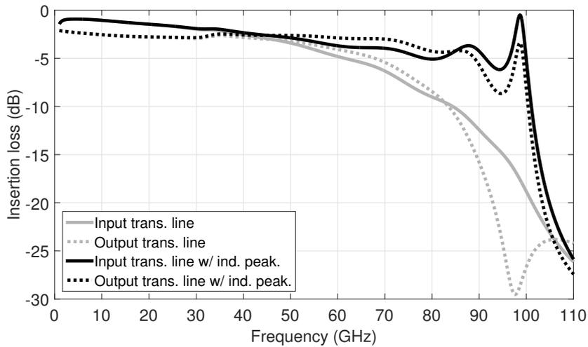
**Figure 5.3:** Simulation of the insertion loss of input and output transmission lines.
