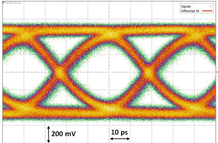
**Figure 4.11:** Measured differential eye-diagram at 25 Gb/s.
