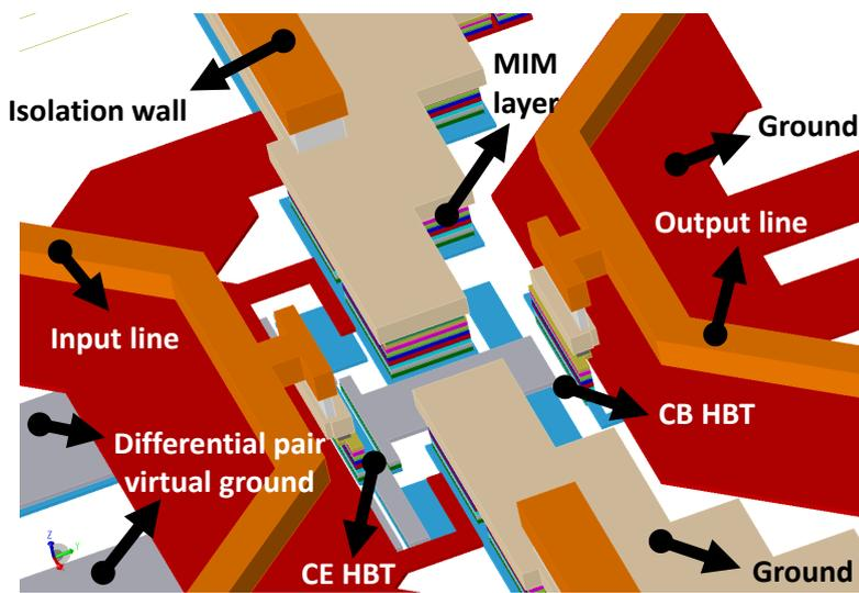
Figure 5.8: Layout 3D view (without resistors and transistors). Layout structure used in electromagnetic simulation in Keysight Momentum.
