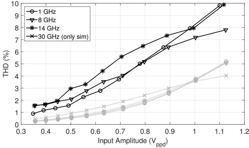
**Figure 5.14:** THD results over input amplitude for different frequency values. Comparison between post-layout simulation (gray) and measurements (black).
