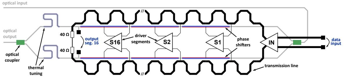
Figure 3.1: Block diagram of the monolithically integrated segmented driver and MZM.
