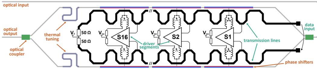
**Figure 3.25:** Block diagram of the second generation monolithically integrated segmented driver and MZM.
