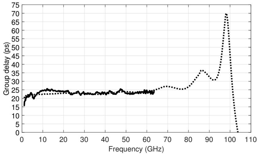
**Figure 5.12:** Differential S-parameters group delay results. Comparison between post-layout simulation (dashed) and measurements (solid).
