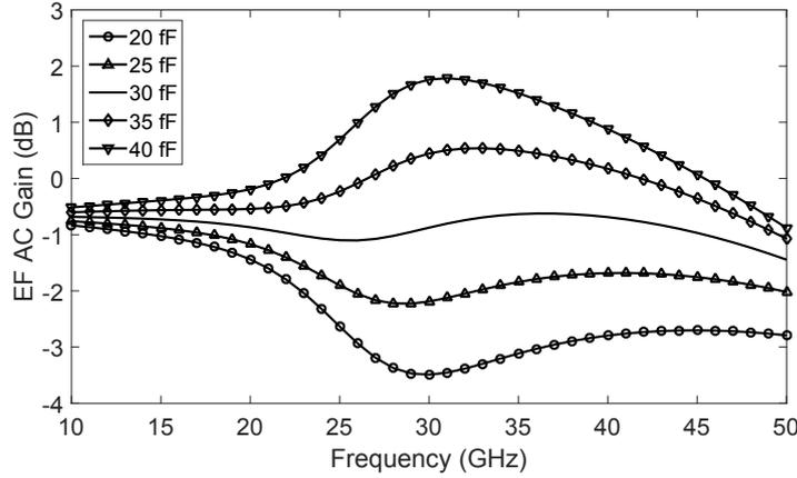
**Figure 3.5:** Simulation of different values of  $C_{neg}$  to determine the negative Miller capacitance value.
