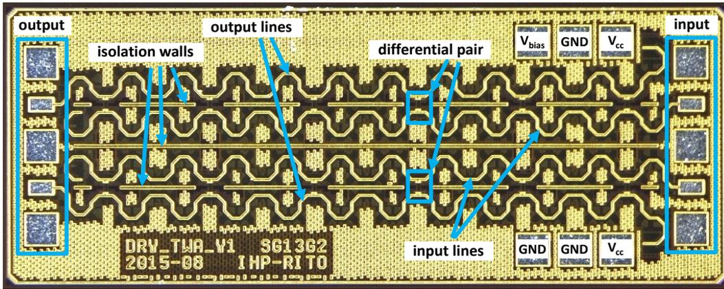
Figure 5.7: Chip microphotograph with pins description and identification of circuit parts.
