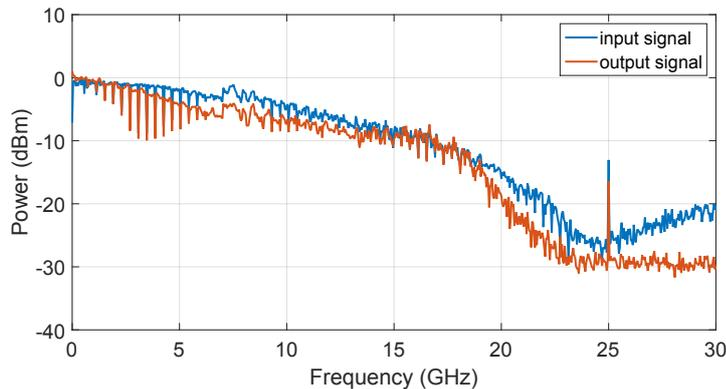
**Figure 3.22:** Spectrum of the optical output in a PAM-4 transmission ( $2^7-1$  PRBS) at 25 Gbaud (50 Gb/s). The spectrum of the input signal is also plotted.
