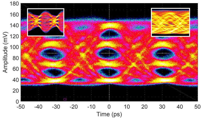
**Figure 3.31:** Electro-optical eye-diagram PAM-4 30 Gbaud (60 Gb/s). The top-left inset shows the input eye-diagram and the top-right inset shows the output eye-diagram without pre-emphasis.
