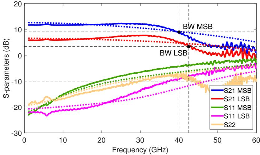
**Figure 4.16:** S-parameters results (gain and return loss). Comparison between post-layout simulation (dashed) and measurements (solid).
