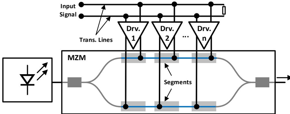
Figure 2.18: Segmented MZM driving scheme.
