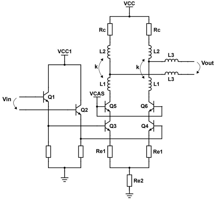
Figure 3.27: Segment schematic of the driver.
