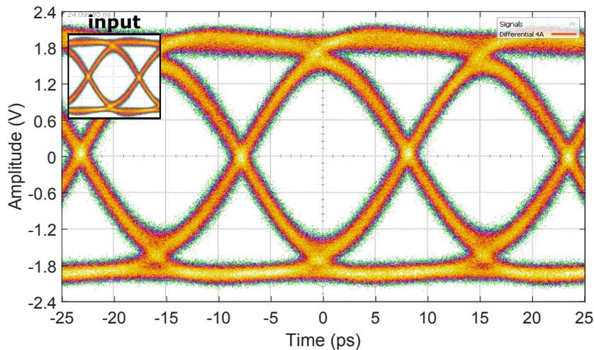
**Figure 5.17:** Differential output eye-diagram OOK 64 Gb/s with  $4 V_{ppd}$  (input  $1.2 V_{ppd}$ ). Measured eye amplitude is  $3.3 V$ , jitter peak-to-peak is  $3.6 ps$  and jitter rms is  $507 fs$ . The inset shows the input eye-diagram.
