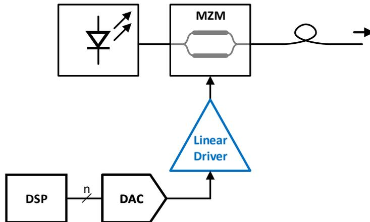
**Figure 1.3:** An electrical driver in an optical transmitter.
