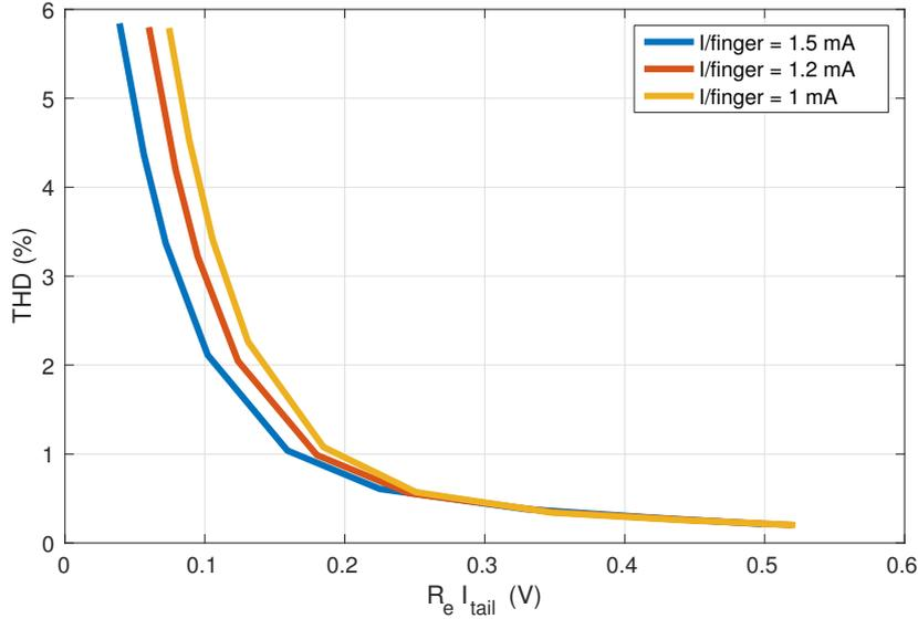
**Figure 2.8:** THD versus  $R_e I_{tail}$  for different current densities per HBT finger.
