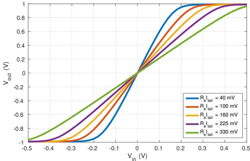
**Figure 2.4:** Output amplitude versus input amplitude for different values of emitter resistance.
