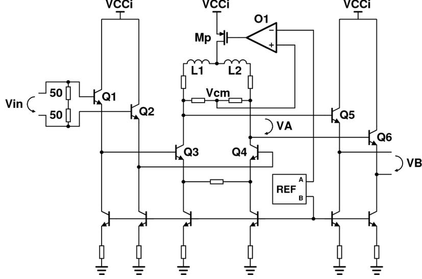
**Figure 4.2:** Detailed schematic of the driver input stage.
