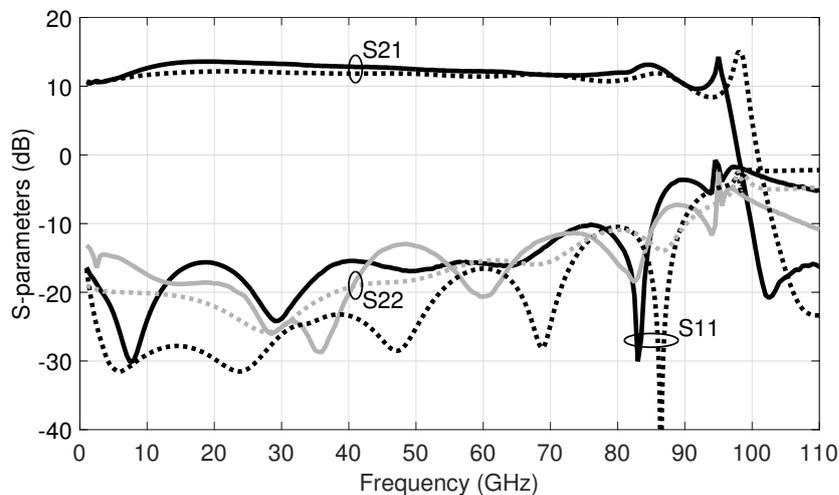
**Figure 5.10:** Single-ended S-parameters results (gain and return loss). Comparison between post-layout simulation (dashed) and measurements (solid).
