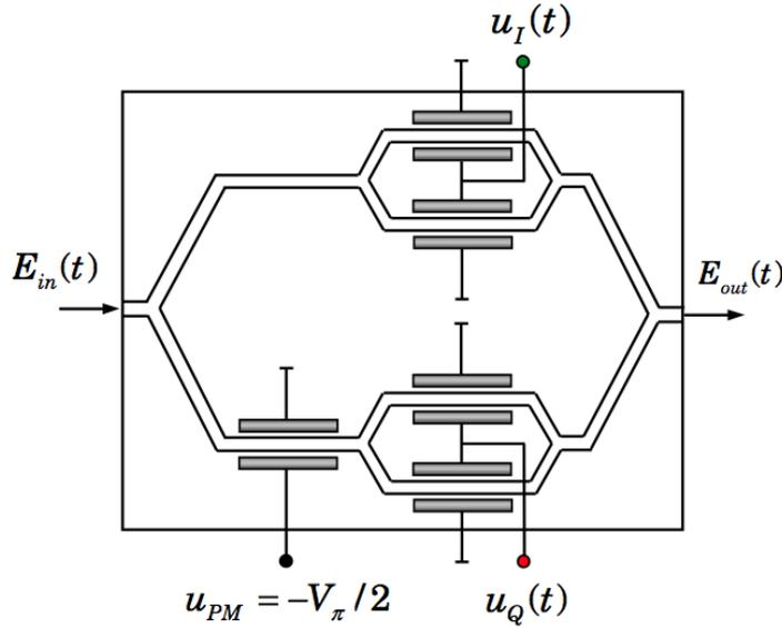
Figure 2.15: Optical IQ Modulator [8].
