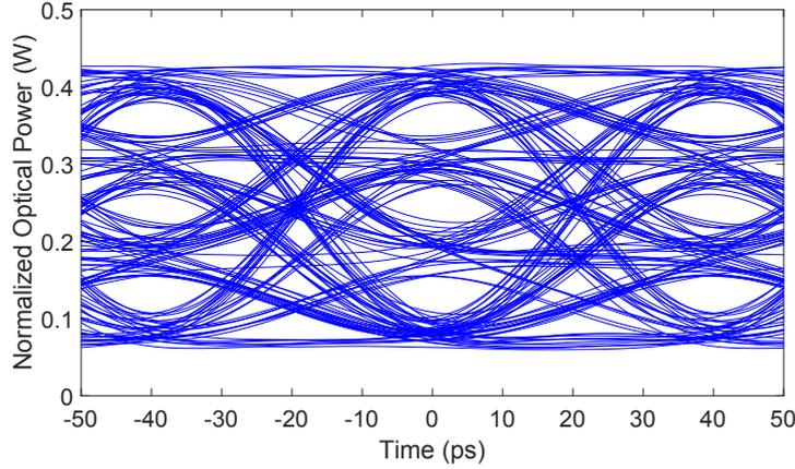
**Figure 3.20:** Simulated optical output eye-diagram transmitting PAM-4 signal at 25 Gbaud (50 Gb/s), using the co-simulation.
