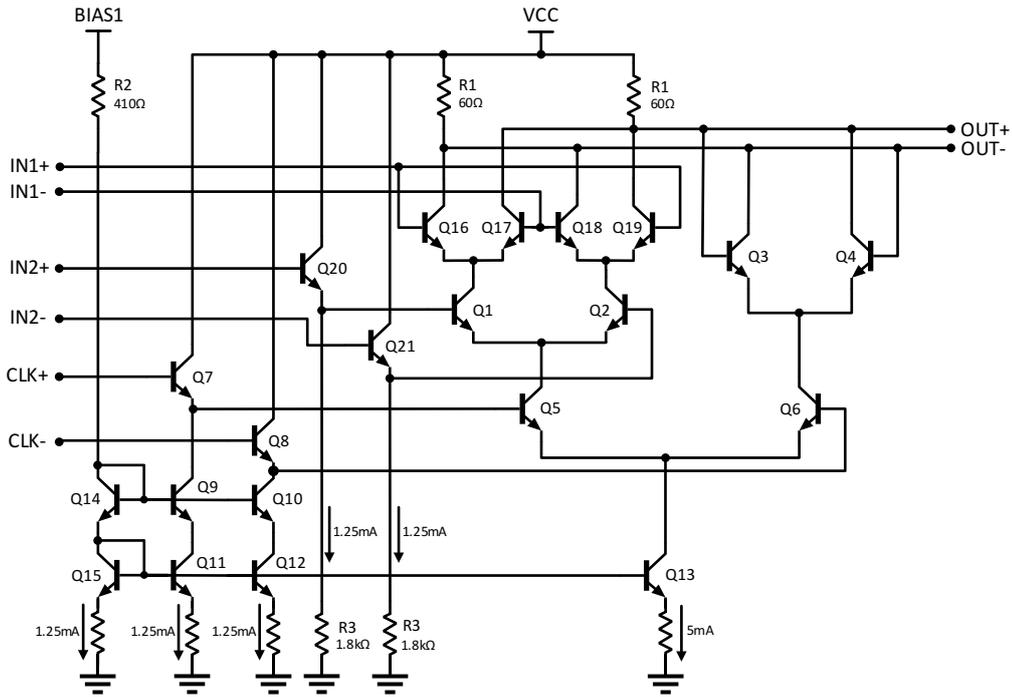
Figure 5.26: Schematic of the latch with XOR function (synchronous).
