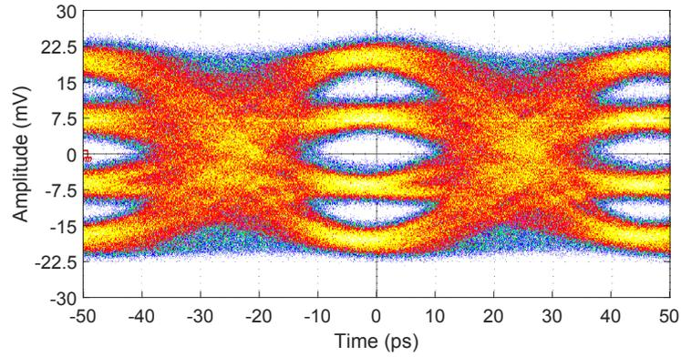
**Figure 3.18:** Measured optical output eye-diagram transmitting PAM-4 signal at 20 Gbaud (40 Gb/s) using  $2^7-1$  PRBS without pre-emphasis.
