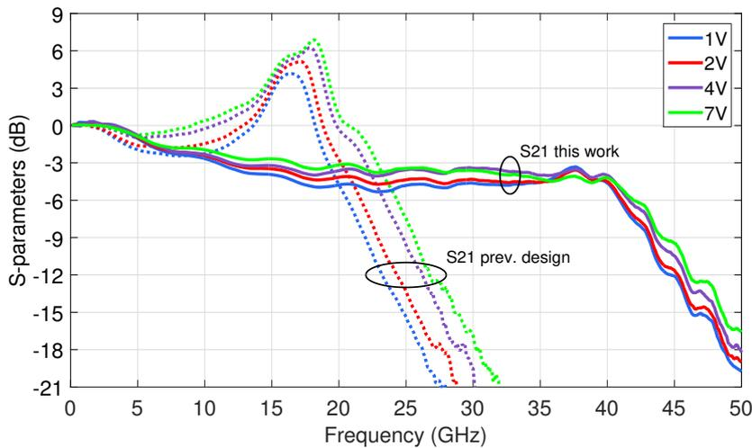
**Figure 3.29:** Electro-optical S-parameters measurements with normalized gain with reverse bias applied to the MZM from 1 V to 7 V.
