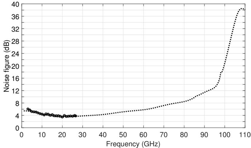
**Figure 5.13:** Single-ended noise figure results. Comparison between post-layout simulation (dashed) and measurements (marked with circles).
