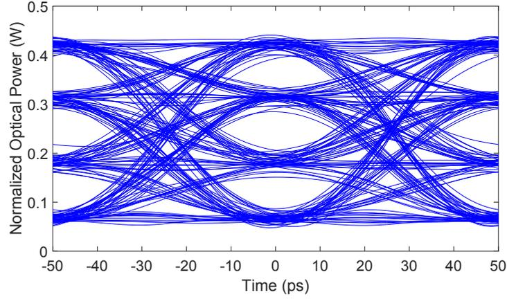
**Figure 3.17:** Simulated optical output eye-diagram transmitting PAM-4 signal at 20 Gbaud (40 Gb/s), using the co-simulation.
