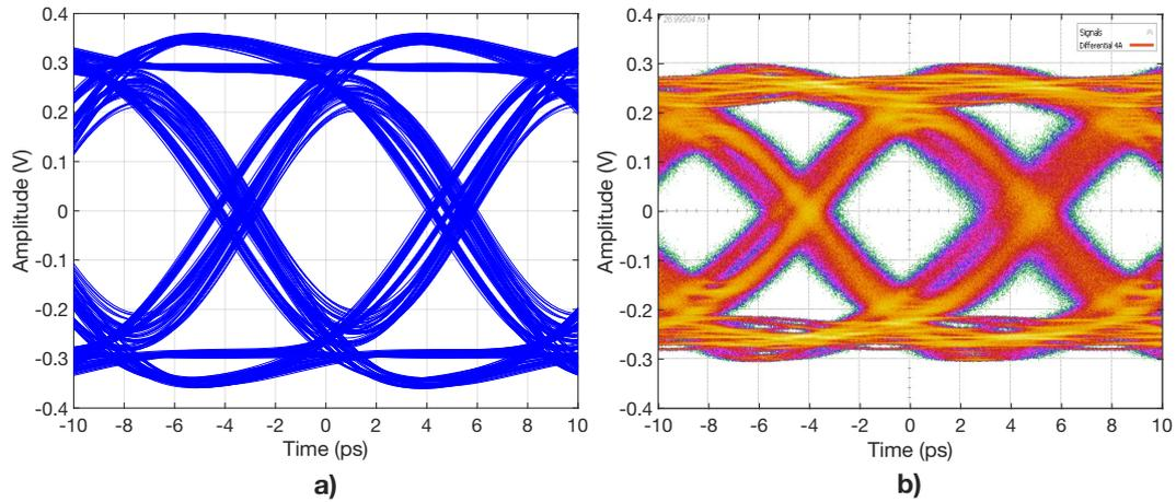
**Figure 5.29:** a) Simulated differential output eye-diagram at 115 Gb/s. b) Measured differential output eye-diagram at 115 Gb/s. The SNR has a value of 5.58 dB, the eye width is 4.97 ps, the eye height is 197 mV and the jitter rms value is 677.6 fs. The acquisition count number is 560.
