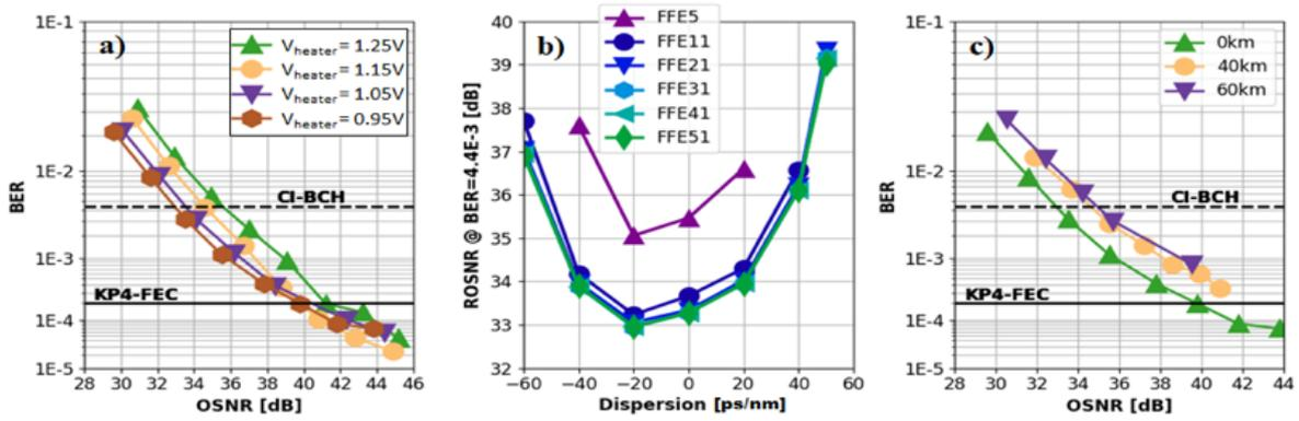
**Figure 3.32:** a) OSNR performance for optical b2b, b) dispersion tolerance and c) OSNR performance at different transmission distances.[51]
