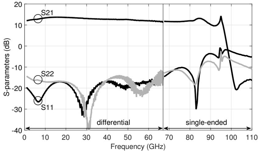
**Figure 5.9:** S-parameters measurement results (gain and return loss).
