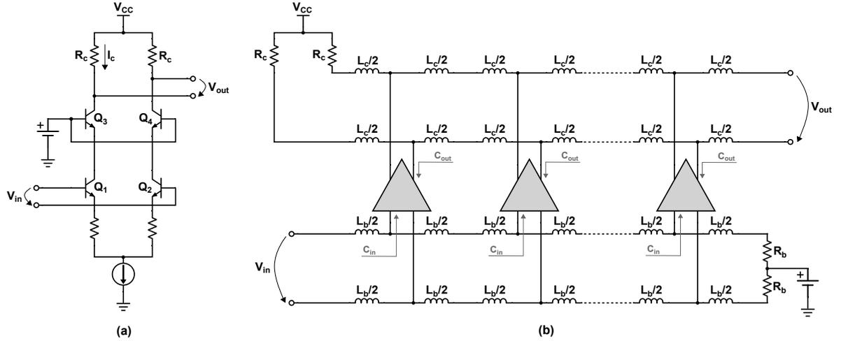
**Figure 5.1:** a) Typical driver schematic. b) Differential distributed amplifier topology.
