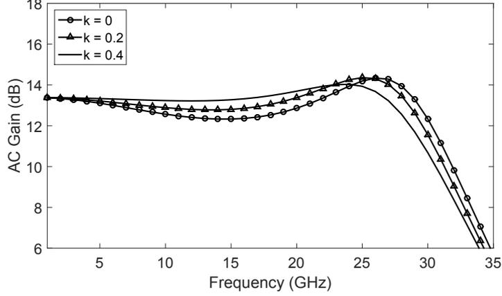
Figure 3.6: Simulation of the effect of coupling in the T-coil design.
