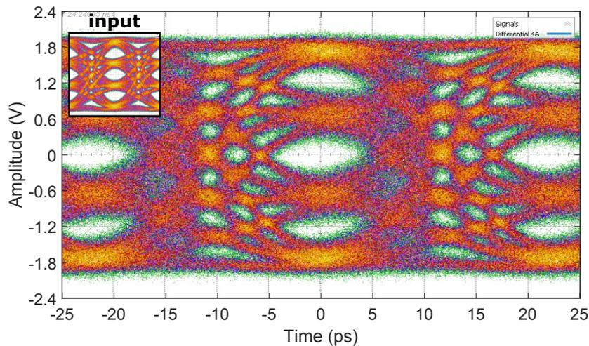
**Figure 5.21:** Differential output eye-diagram PAM-4 45 Gbaud (90 Gb/s) with  $4 V_{\text{ppd}}$  (input  $1.2 V_{\text{ppd}}$ ), without pre-emphasis. The inset shows the input eye-diagram.
