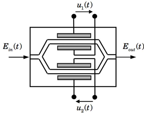
**Figure 2.13:** Integrated optical Mach-Zehnder modulator (dual-drive) [8].
