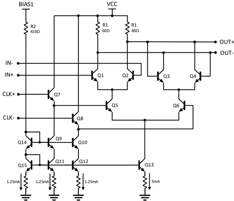
Figure 5.24: Schematic of the standard latch.
