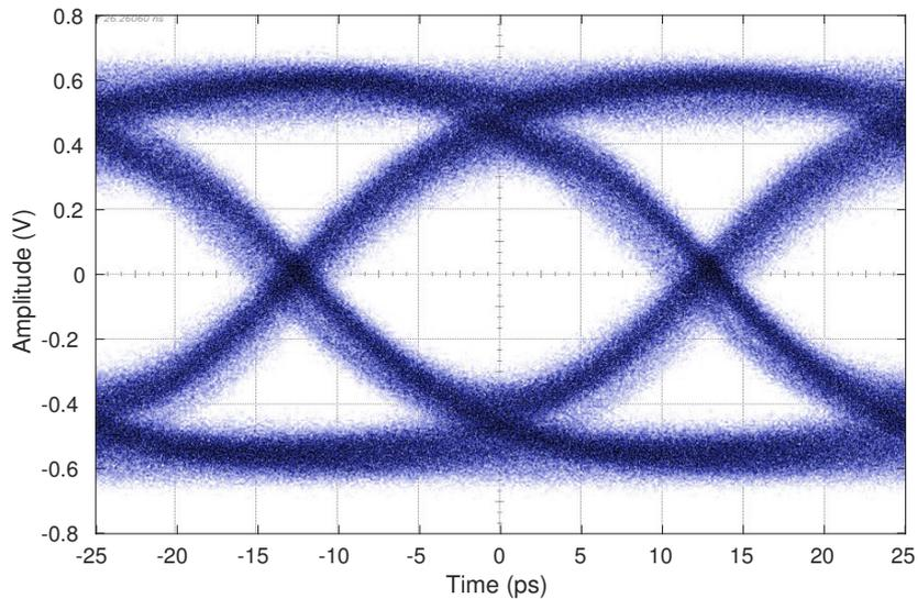
**Figure 4.6:** Differential output eye-diagram at 40 Gb/s. Signal is attenuated by 10 dB at the input of the oscilloscope. Input amplitude is limited to 1.2 Vppd.
