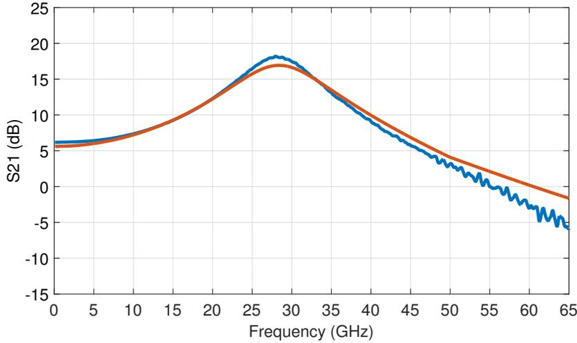
**Figure 3.28:** Comparison of simulated (red) and measured (blue)  $S_{21}$  of the driver with one segment.
