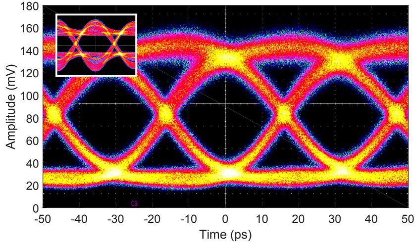
**Figure 3.30:** Electro-optical eye-diagram OOK 34 Gb/s. The inset shows the input eye-diagram.
