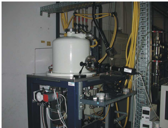
Figure 3.5: Photography of the apparatus that was used for mPD growth experiments.
