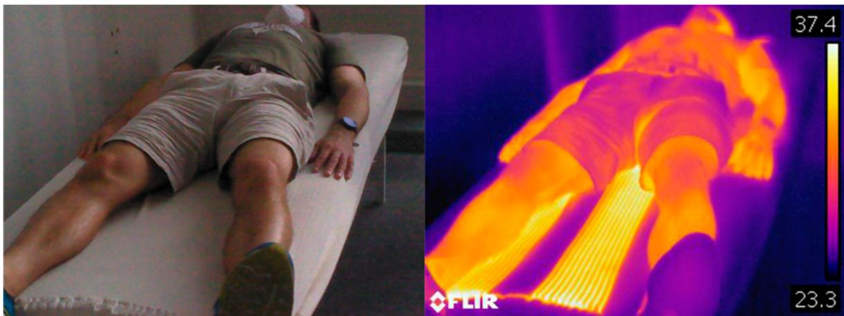
**Figure 22.** A 90 cm × 190 cm knitted bed sheet with integrated Y08 yarns, ultrasonically welded with conductive ribbon Elasta Vestil as a continuous contact element for the interconnection of the heating yarns.
