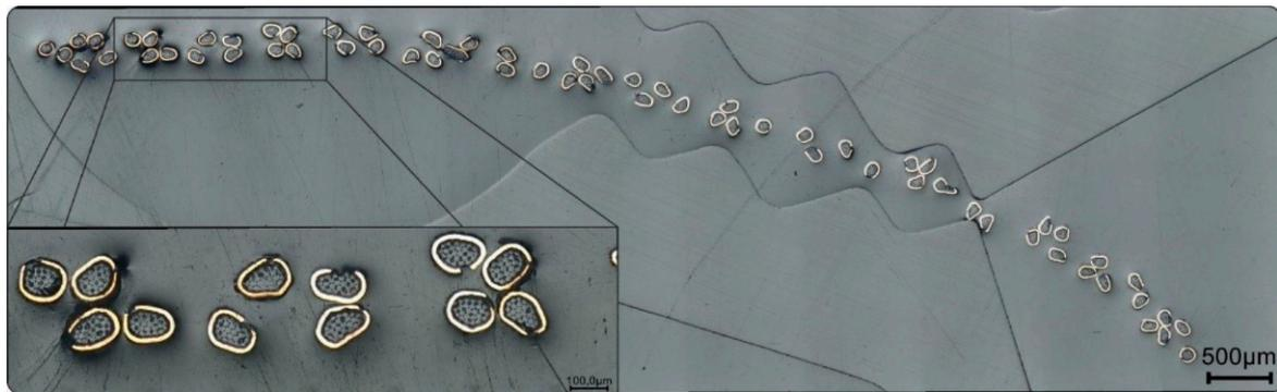
**Figure 5.** Cross-section image of the High Flex 3981 braided ribbon. In the zoom window, the individual yarns covered with thin silver-plated copper foil are shown for better visualization.
