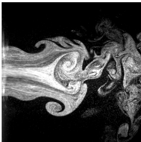
Figure 1.2: Smoke visualization of a laminar swirling jet ( Re = 1200 ) undergoing vortex breakdown. Source: [107].
