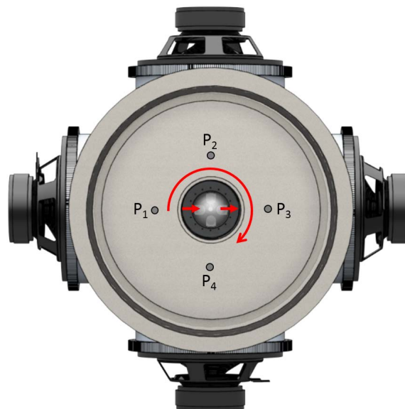
Figure 1.13: Circumferential sensor arrangement ( P_1 - P_4 ) with azimuthal actuation direction ( m = 1 ) indicated by rounded arrow. Small red arrows exemplary indicate actuation jets generated by the four loudspeakers in the background. (View onto the burner front plate from the downstream end of combustion chamber)
