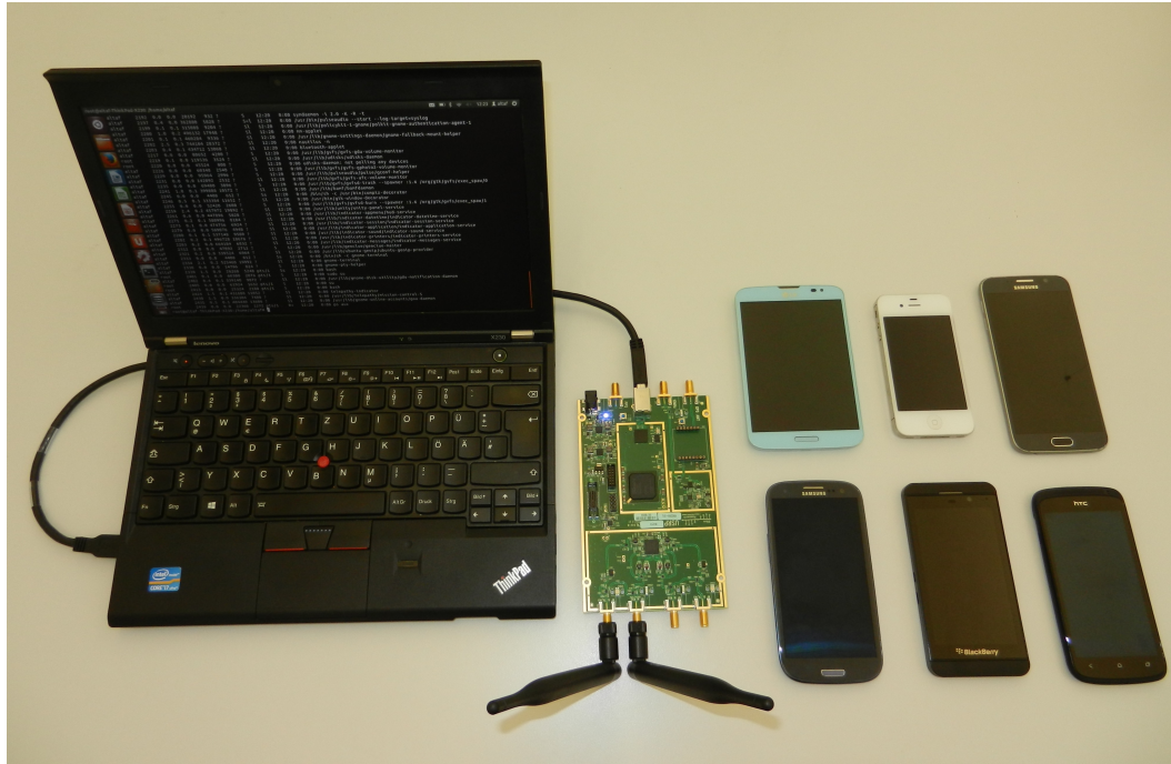
Fig. 3.2.: Passive listener and Rogue eNodeB
