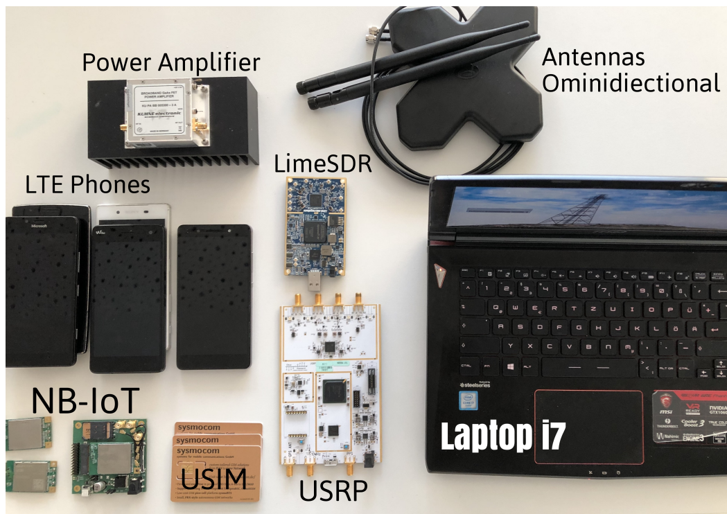
Fig. 3.1.: Low-cost Hardware Components for LTE network operation
