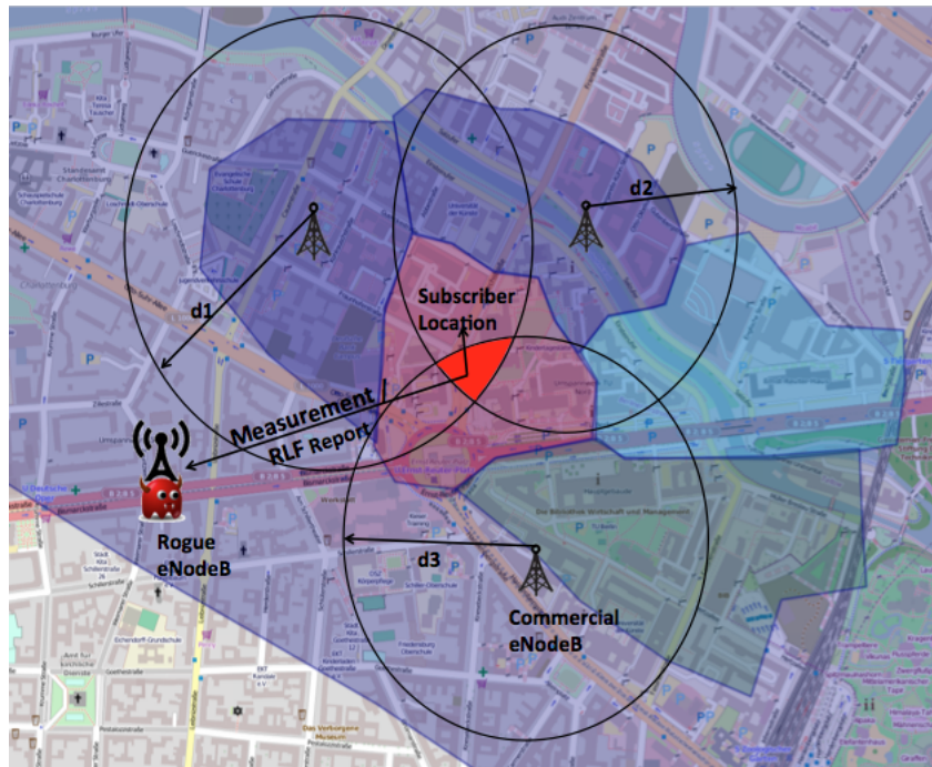
Fig. 4.4.: Determining subscriber's precise location using trilateration (L3)
