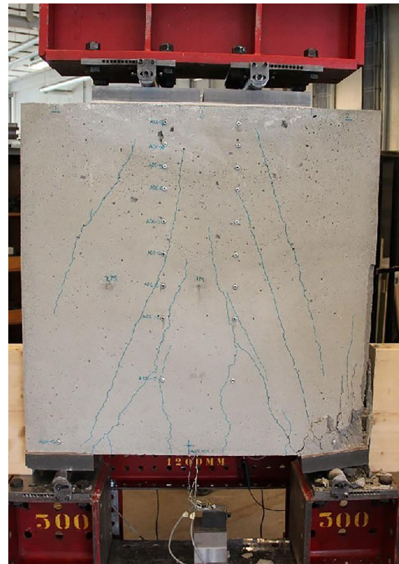
FIGURE 4 Bearing failure of Infra lightweight concrete wall beam [81]
