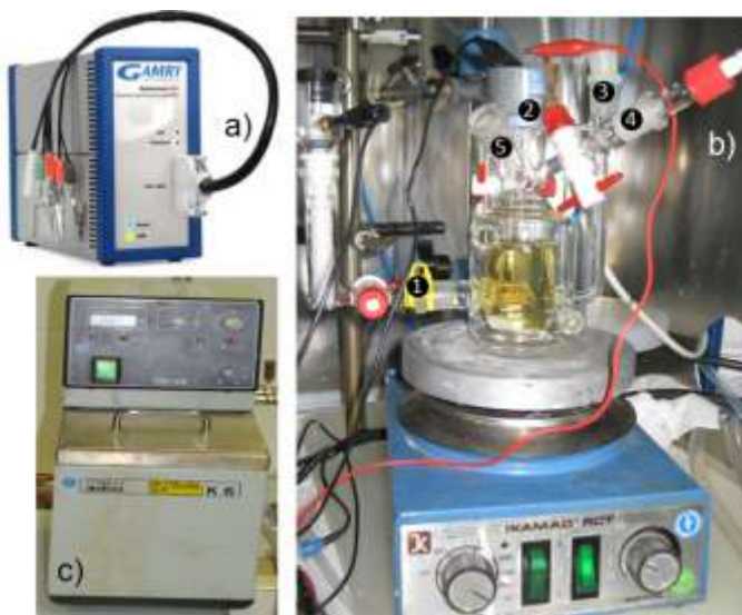
Fig. 2. 5 Three electrode electrochemical cell setup; a) Gamry reference potentiostat 600 series; b) electrochemical cell with five provisions on magnetic stirrer; c) hot water circulation for heating the cell.
