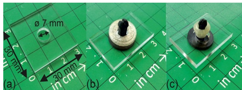
Figure 4.2.2. A one-time active assembly is enabled by heating the 4D-printed round disk made from PPG-based PEU. A poly(methyl methacrylate) sheet with an opening in the middle (a), fastener pin, and round disk were placed together with the sheet (b) and assembled by heating the round disk to 75 °C (c).
