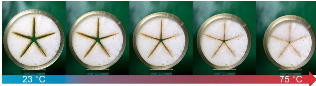
Figure 4.2.12. Thermomechanical treatment of PEUU foam with a star-shaped cutout using a 4D-printed cylinder made of PEU. The temperature was systematically raised from 23 °C to 75 °C (from left to right).
