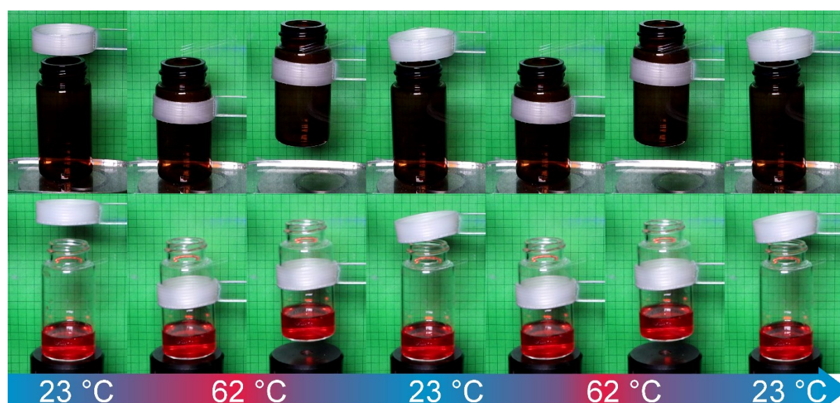
Figure 6.11. 2W 4D-printed cylindrical actuators of PDA-based PEU in operation: Gripping, lifting, releasing of (top row) an empty brownish vial (15 g in weight) and (bottom row) a transparent vial filled with red liquid (total weight of 30 g) in two consecutive thermal cycles.
