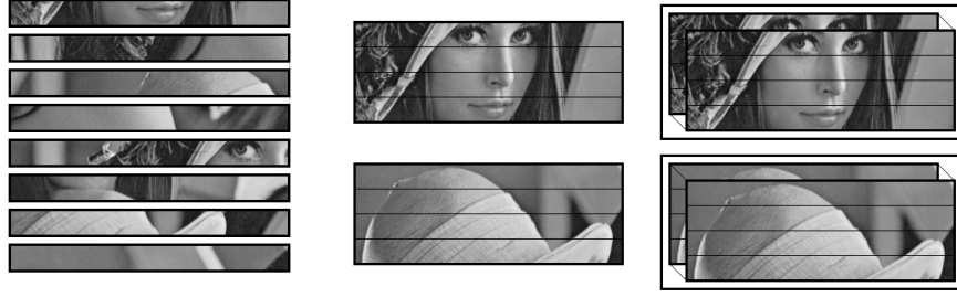
(a) Eight 1D MDSC blocks. (b) Two 2D MDSC blocks, four lines high. (c) Two 3D MDSC blocks, four lines high and 2 images deep.
