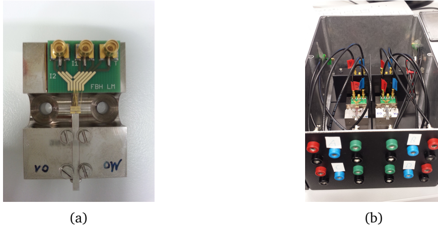
Figure 5.4: Submount holder with electrical interface and a 3 mm DFB mounted (a), and an open burn-in box for four submount holders (b)
