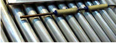
Figure 2.6: Installation of a PT-100 element inside an SWHE bundle (from Reithmeier et al. , 2004/04/21-24)
