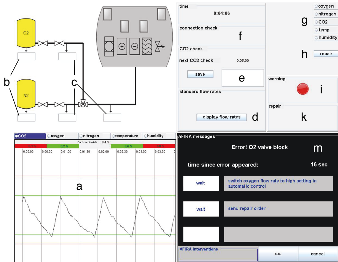
Figure 2.1: AutoCAMS 2.0 User Interface with activated Action Implementation Support. The figure shows the following elements of the AutoCAMS 2.0 User Interface: (a) monitors / history graphs for each subsystem, (b) O_2 and N_2 tank level readings, (c) O_2 , N_2 and mixer valve flow readings, (d) standard flow rates, (e) input field for CO_2 readings (secondary task), (f) connection check icon (secondary task), (g) menu for manual control of each parameter, (h) menu for repair orders, (i) master alarm, (k) repair order information, (m) automated aid (Automated Fault Identification and Recovery Agent, AFIRA).
