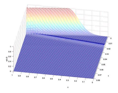
Figure 12: Time evolution of  $|\psi_a(x,t)|$ : The approximate convolution coefficients consisting of L = 10 discrete exponentials give rise to a reflected wave.
