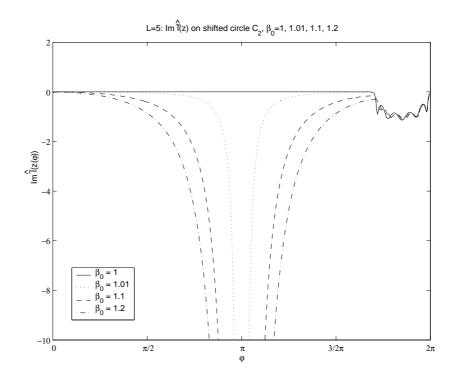
Figure 10: Stability condition Im  $\tilde{\ell}|_{\mathcal{C}_2} \leq 0$  for exponential-sum-coefficients with L = 5. The condition is not satisfied for  $\beta_0 = 1$  but is satisfied for  $\beta_0 \geq 1.00025$ .
