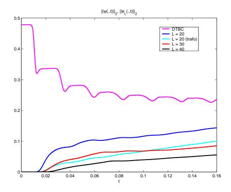
Figure 17: Time evolution within the potential well (V = 4500) of the discrete  $\ell^2$ -norm  $\|\psi(.,t)\|_2$  and of the errors  $\|e_L(.,t)\|_2$  that are due to approximated DTBCs with L = 20, 30, 40. "L = 20 (trafo)" uses convolution coefficients calculated by the Transformation 3.1.
