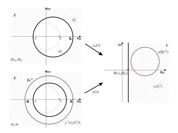
Figure 7: Illustration of the 2 maps  $y_0(z)$  and y(z) from the proof of Theorem 5.1: The circle  $z = \beta e^{i\varphi}$  (dashed line) is mapped onto  $y(\beta e^{i\varphi})$  which lies inside the (shaded) stability region  $y_0(\mathcal{C}_1^o)$ .
