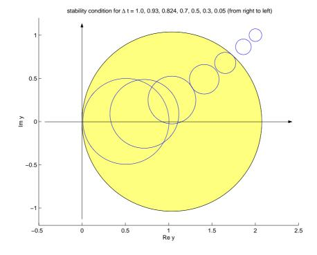
Figure 8: Illustration of the proof of Theorem 5.2 (b): For  $\Delta t \leq \Delta t_1 \approx 0.82$ the (small) circles  $\{y(\Delta t, \varphi) \mid 0 \leq \varphi \leq 2\pi\}$  are inside the (shaded) stability region  $y_0(\mathcal{C}_2^o)$ . Parameters:  $\Delta x_0 = \Delta t_0 = V = \gamma = 1$ ,  $\rho = 4$ .
