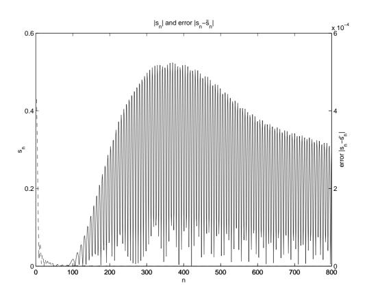
Figure 3: Convolution coefficients  $s_n$  (left axis, dashed line) and error  $|s_n - \tilde{s}_n|$  of the convolution coefficients (right axis);  $\Delta x = 1/160$ ,  $\Delta t = 2 \cdot 10^{-5}$ , V = 0 (L = 20)
