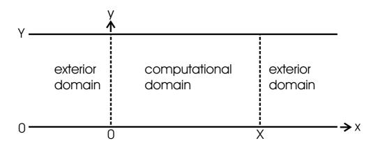
Figure 1: The artificial BCs at x = 0, x = X cut off the exterior domains.
