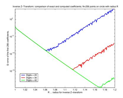
Figure 2: Relative error of the numerical inverse Z-transform of  $\hat{s}$  depending on  $\rho$  (the radius of the integration circle) for different values of Digits (the mantissa length). The three curves overlap exactly on the decaying branch, and their increasing branches – corresponding to the amplified round-off error – are 10 orders of magnitude apart. Here  $\Delta x = 1/160$ ,  $\Delta t = 2 \cdot 10^{-5}$ , N = 256.
