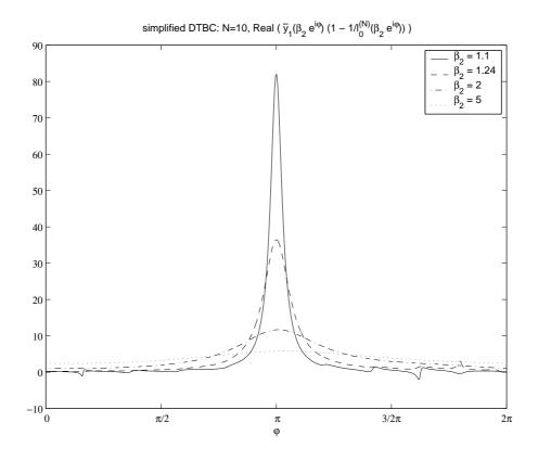
Figure 11:  $h^1$ -condition (6.14a) for simplified discrete transparent boundary conditions with cut-off after N = 10 convolution coefficients,  $\Delta x = 1/160$ ,  $\Delta t = 2 \cdot 10^{-5}$ ,  $V \equiv 0$ . The  $h^1$ -condition (6.14a) is satisfied for  $\beta_2 \geq 1.24$ .
