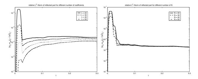
Figure 14: Error of the approximate solution  $\psi_a(t)$  with (a) approximate convolution coefficients consisting of L = 20, 30, 40, 50 discrete exponentials; (b) "cut-off" DTBC: The convolution coefficients are cut off for  $n \ge N$  with N = 20, 30, 40, 50. The error-peak between t = 0.01 and t = 0.02 corresponds to the first reflected wave, which is clearly visible in Figure 12.
