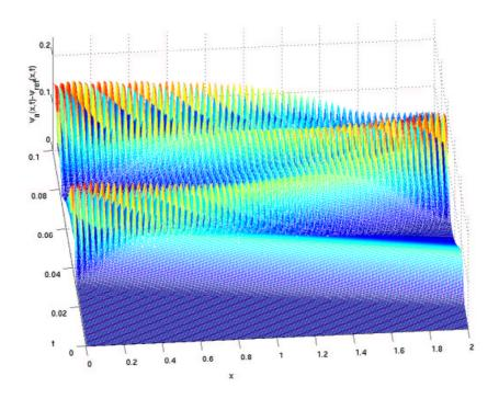
Figure 16: Time evolution within the potential well (V = 4500) of the error  $|e_L(x,t)|$  due to an approximated DTBC with L = 20. As expected, the error accumulates with each reflection of the main wave.
