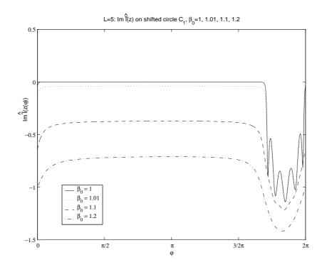
Figure 9: Stability condition Im  $\tilde{\ell}|_{\mathcal{C}_1} \leq 0$  for exponential-sum-coefficients with L = 5. The condition is not satisfied for  $\beta_0 = 1$  but is satisfied for  $\beta_0 \geq 1.0000008$ .
