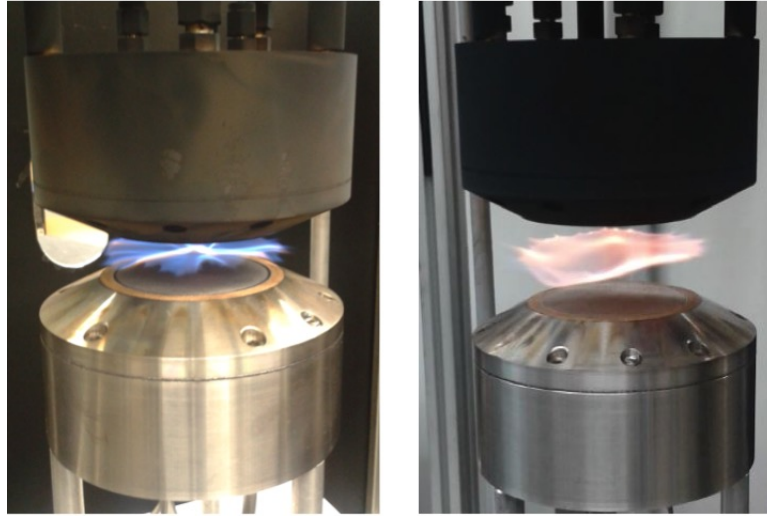
Figure 5.2: Diffusion flames at L/D = 0.36 (left) and L/D = 0.83 (right) [23] induced by two opposed McKenna flat flame burners
