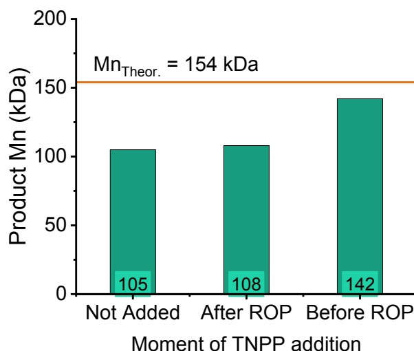
Figure 5.31: Changes in the copolymer Mn depending on the moment of TNPP addition. All copolymers had a 13 %-wt PEPG20 content, a 4 %-wt D-lactide content and 0.35 %-wt TNPP content with a theoretical Mn of 154 kDa according to the given [lactide] / [-OH] ratio.
