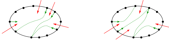
Figure 4.10: Adding help-edges in a face. The flow \psi is depicted by red arcs. The green half-arcs together with the dashed extensions represent the help-edges.
