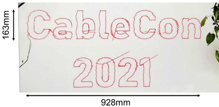
Figure III.18: Text as an example of the accuracy in the horizontal and vertical directions of the robot
