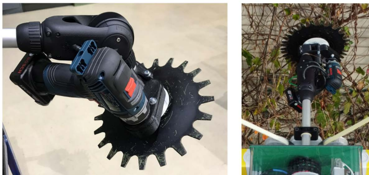
Figure III.23: Modified rotary scissor tool head for cutting thin branches and leaves (images by Sebastian Schröder)
