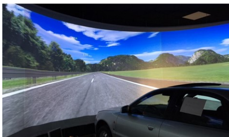
Fig. 1. The driving simulator at the Department of Automotive Engineering at Technische Universität Berlin, Germany.
