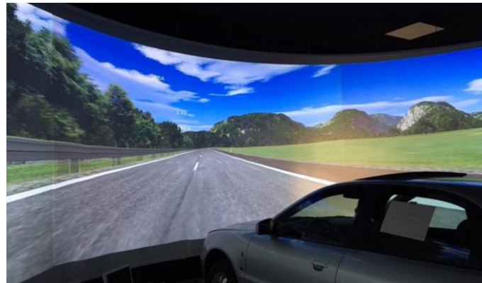
Fig. 1. The driving simulator at the Department of Automotive Engineering at Technische Universität Berlin.
