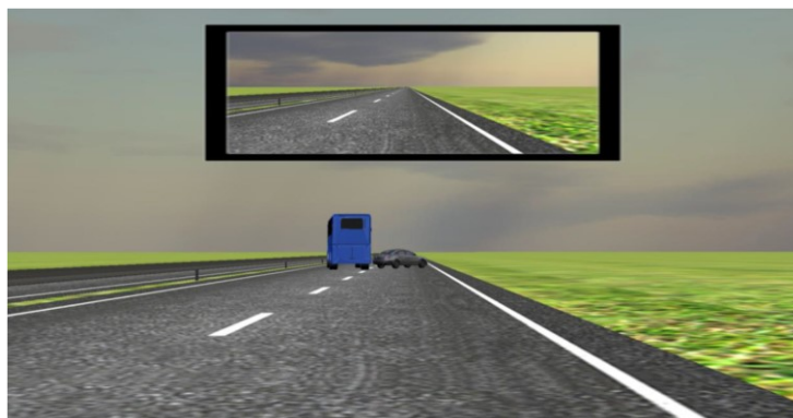
Fig. 3. Take-over situation with 2.5 s TTC, the crashed vehicle in grey (right), and the lead vehicle in blue (left). The rectangle in the upper-middle represents the rear-view mirror.
