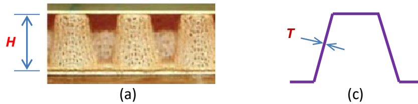
Fig. 7. Geometrical parameters of the nap-core: (a) height H ; (b) fabric thickness T .
