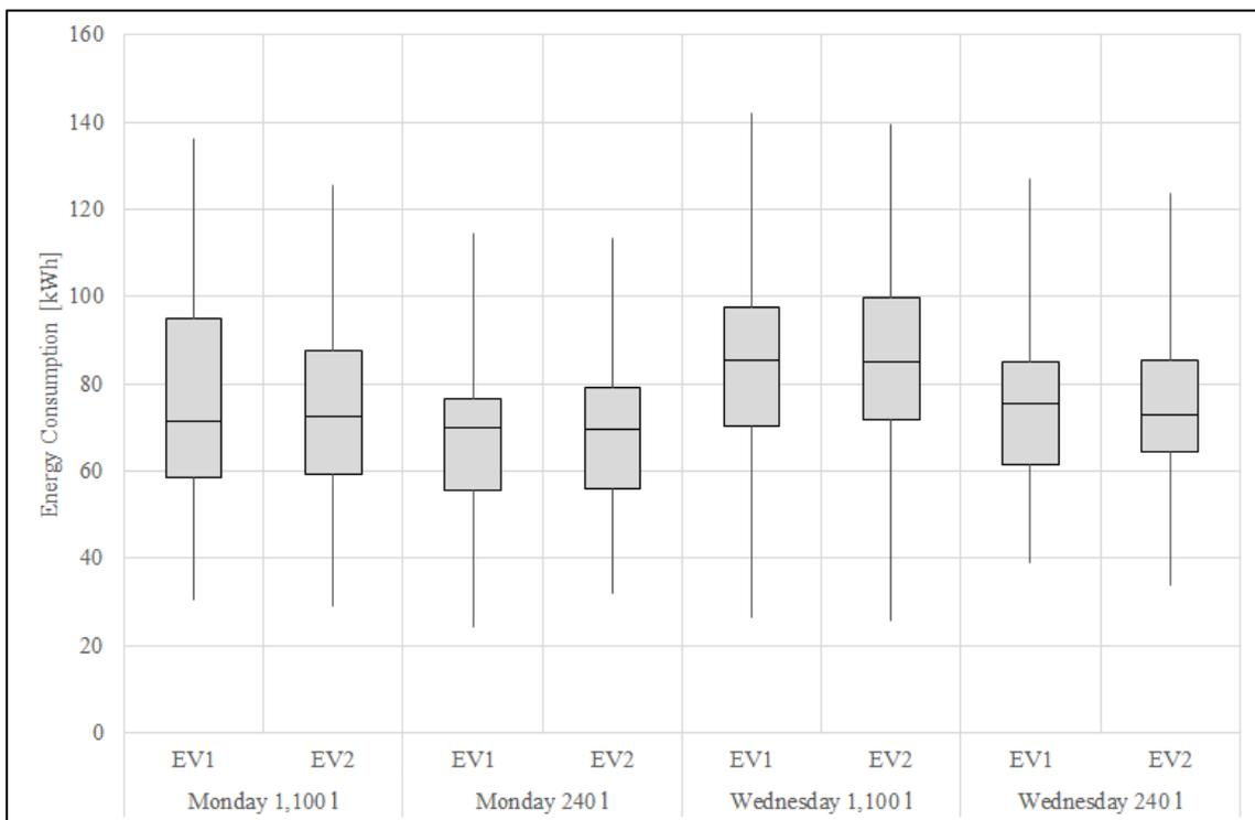
Figure 4: Distribution of energy consumption per tour and vehicle for the different simulation setups
