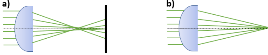
Figure 2.2: Light rays passing through a) a spherical lens and b) an optimized aspherical lens.
