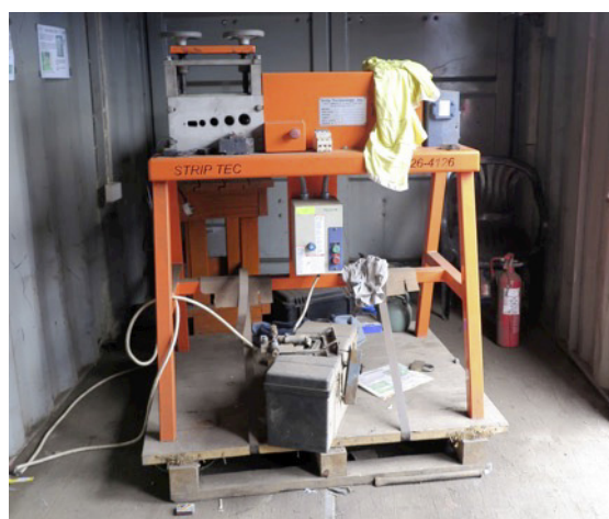
Figure 5. One of the cable-stripping machines. © SMART/Maja van der Velden.
